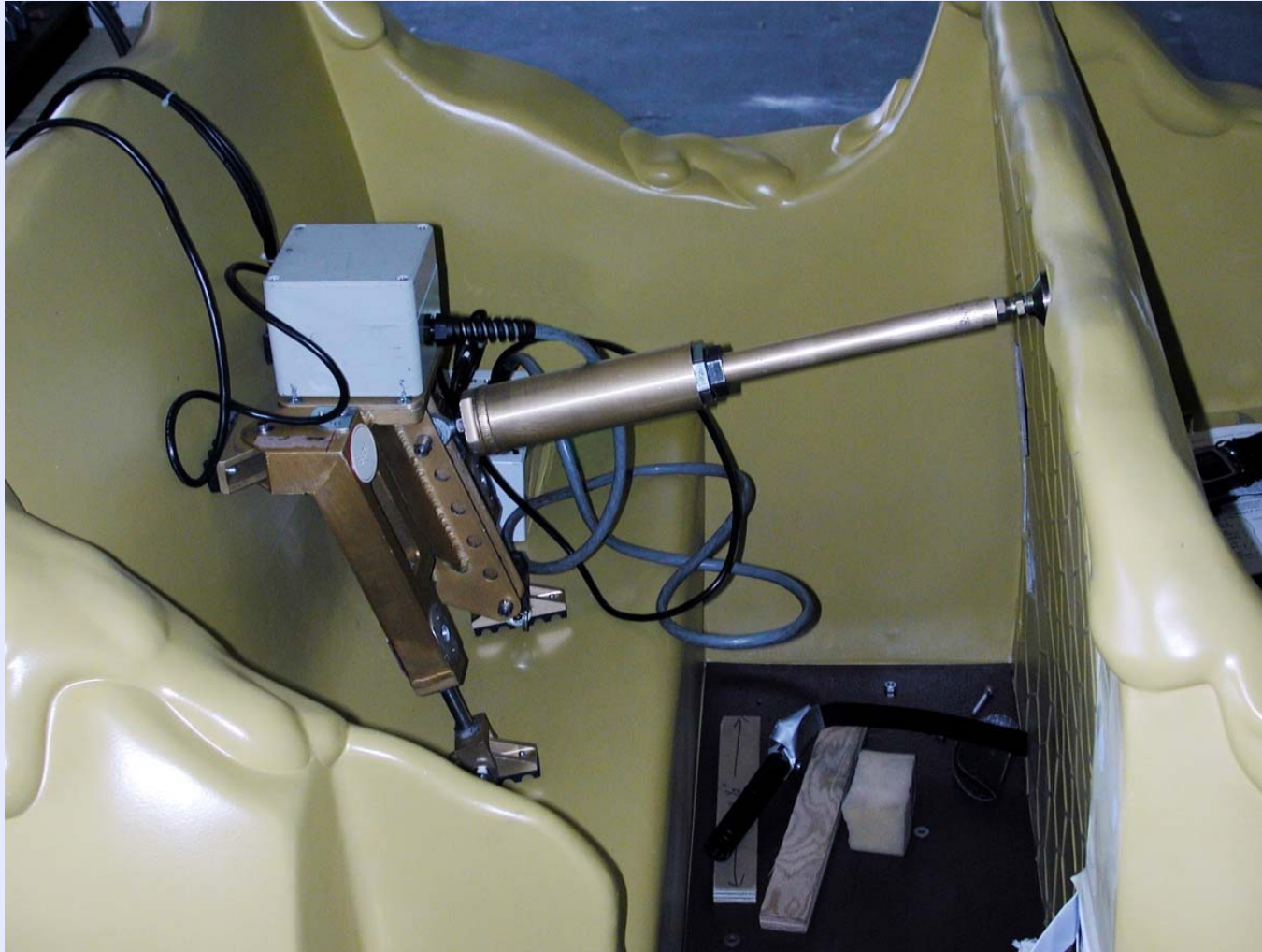
Fixed Placement of Accelerometer, Standardized Collection
