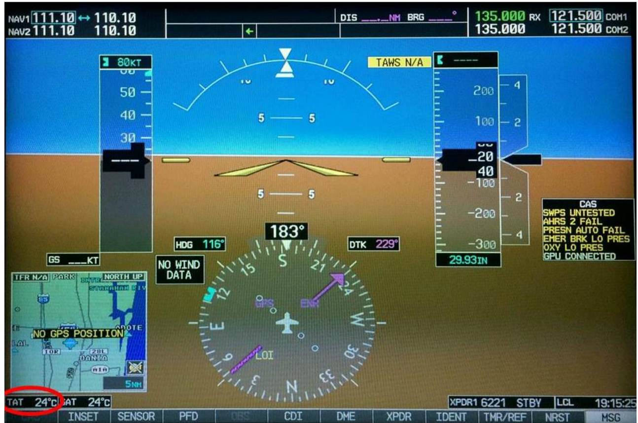
Figure 2. The TAT display (circled in red) as shown to EMB-500 pilots in normal operation.
