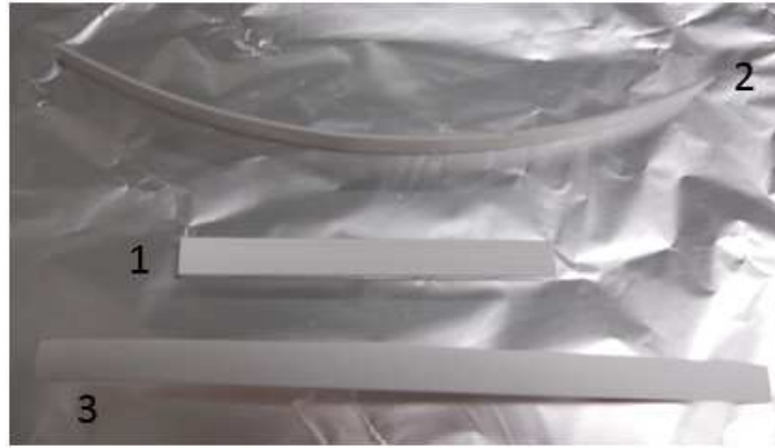
Figure 6.17: Picture of the Al samples tested for the high vacuum compatibility. Sample 1: rectangle of 10 cm × 1 cm × 0.5 cm, with etched grooves for the wire winding. Sample 2 and 3: ring section - curved length about 21 cm, width = 1 cm, height = 1.5 mm. Coating thickness is 0.10 mm for samples 1 and 2 and 0.15 mm for sample 3. The maximum voltage applicable to this coating is about 140 V/ 0.1 mm.
