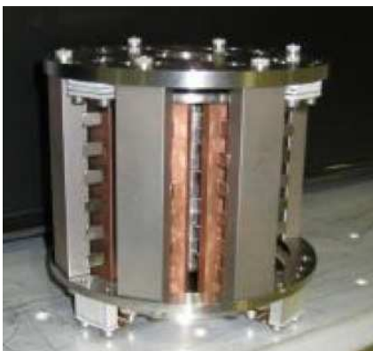
Figure 12.15: (left) Picture of one of the three vertical eddy current damper used to reduce the quality factor of the vertical spring box modes. (right) Damping of the 34.5 Hz tilt mode of the spring box. About 20 dB suppression has been achieved.
