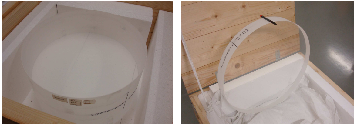
Figure 5.1: Input Mirror Blank (35 cm diameter, 20 cm thick, left), BS blank substrate (55 cm diameter, 6.5 cm thick, right)
