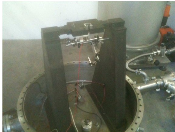
Figure 10.17: The Perugia test facility for violin modes Q measurements.
