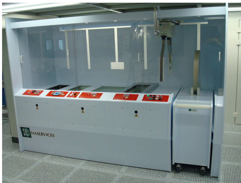
Figure 5.8: New wet cleaning machine needed for AdV installed in the clean room.
