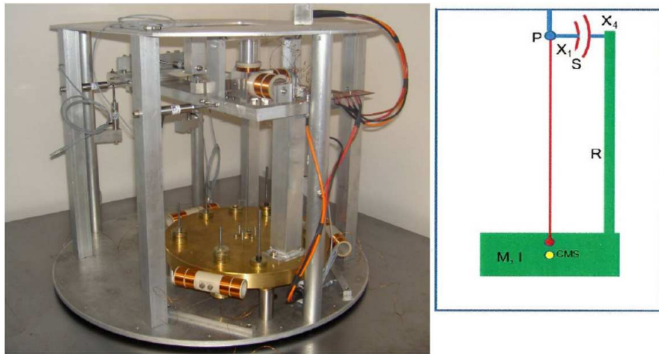
Figure 11.38: Left: Image of the new tiltmeter prototype assembly. Right: Scheme of its basic working principle: sensing is realized by means of a spherical sensor S measuring the relative displacement x_1 - x_4 . The horizontal acceleration of the box induces a sensor S output that is, to the first order in the box tilt angle, insensitive to box tilts.
