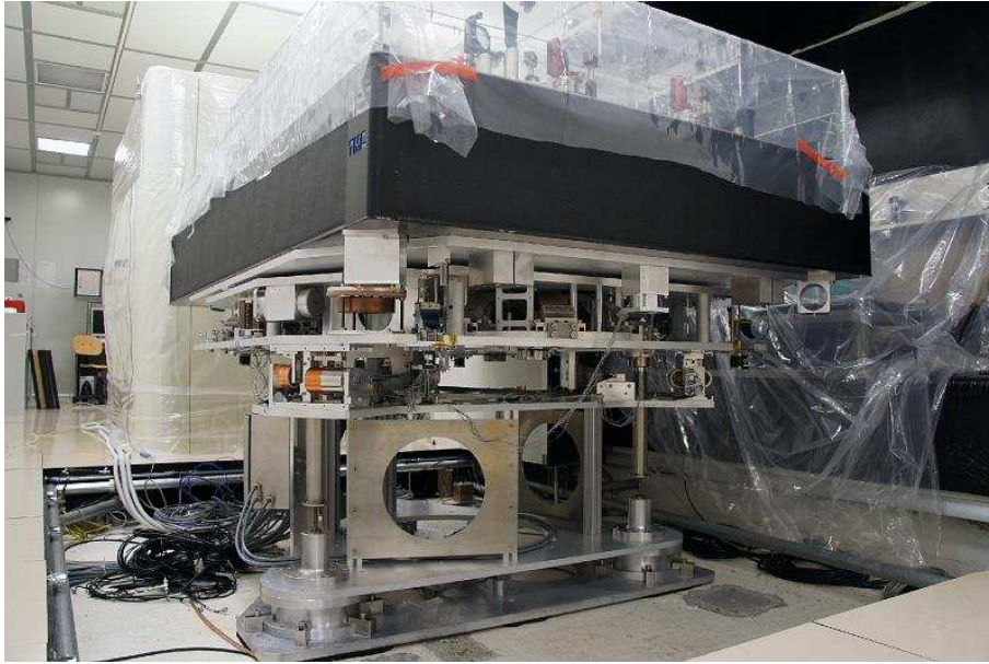
Figure 12.2: EIB-SAS as installed in the Virgo LLab.
