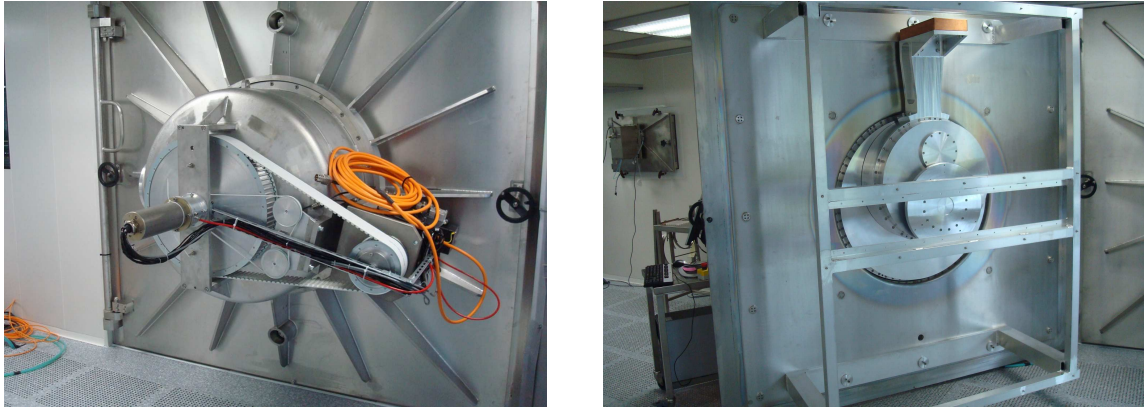
Figure 5.5: Pictures of the new robot for the CC installed on the Virgo coating chamber.
