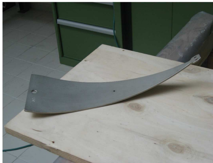
Figure 11.28: A pre-bent blade
