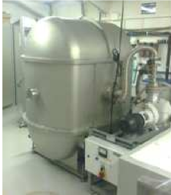
Figure 10.19: The Rome vacuum chamber for payload testing.
