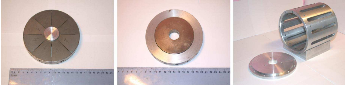
Figure 4.52: Components of the magnetic system of the AdV isolator prototype. Left: composite rings with radial direction of the magnetization vector. Center: monolithic ring with axial direction of the magnetization vector. Right: aluminium case used to mount the assembly of magnetic rings.
