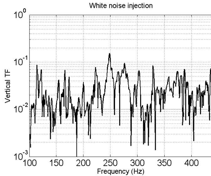
Figure 12.20: Ground-to- EIB vertical transfer function.
