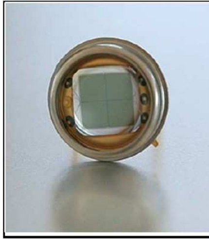
Figure 7.15: QP45-Q by First Sensor features 4 quadrants with 11 mm 2 surface area. The gap that separates the sensitive regions amounts to 70 \mu\text{m} .
