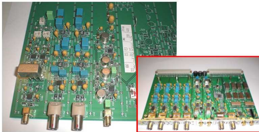
Figure 7.17: Prototype board that is used to demodulate signals from quadrant photodiodes in Advanced Virgo for frequencies up to 200 MHz. The insert shows a demodulated board developed for Virgo+.
