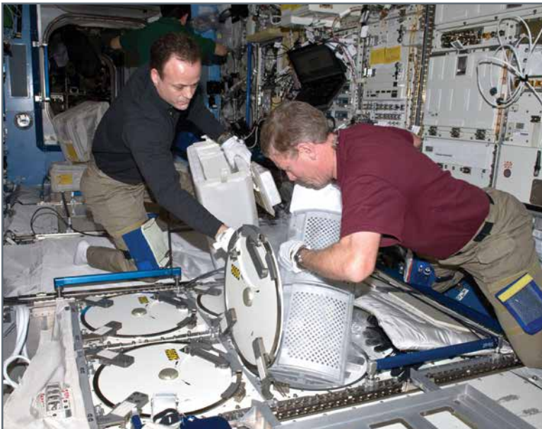
ISS crewmembers Ron Garan (left) and Mike Fossum remove samples from GLACIER and insert in the MELFI-1 in the Kibo laboratory of the ISS (ISS028E014916).
