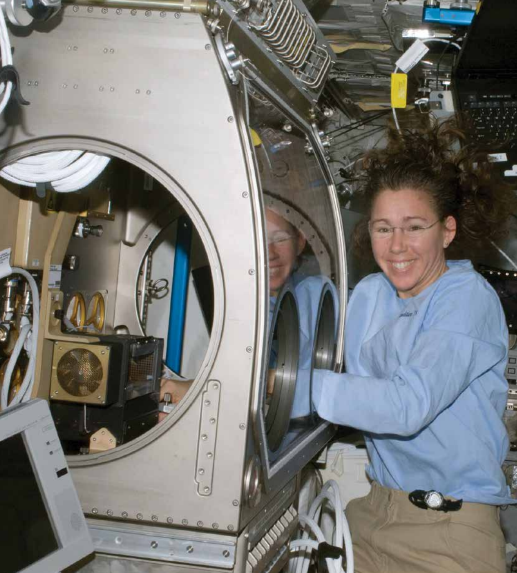
Astronaut Sandra Magnus works with the Smoke Point In Co-flow Experiment (SPICE) using the Microgravity Science Glovebox (MSG) during Expedition 18 (ISS018E026974).
