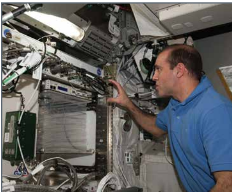
ISS crewmember Rick Mastracchio installs the Veggie hardware into EXPRESS Rack 3 (ISS039E019105).
