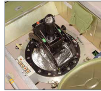
Russian experiment Fialka multispectral ultraviolet system hardware installed on the Service Module/Zvezda window (ISS015E28944).
