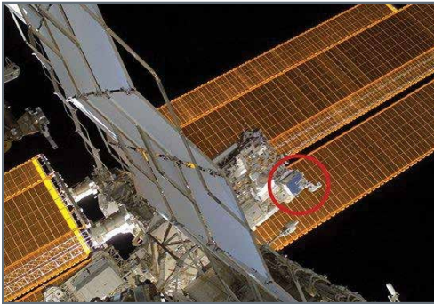
External image of the ISS showing SCAN Testbed installed on ELC 4 nadir side (NASA).
