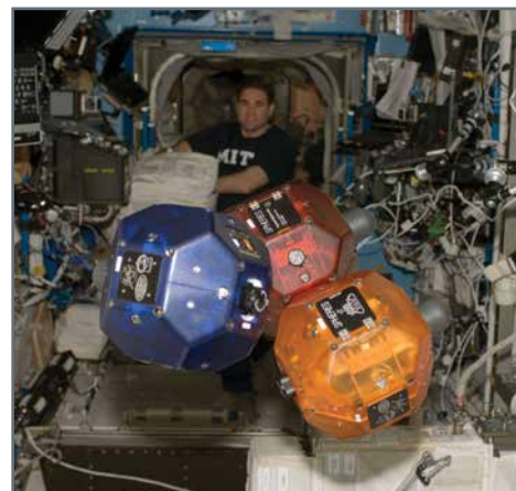
Astronaut Greg Chamitoff programming a SPHERES test run during Expedition 17 and 18 (ISS018E005212).
