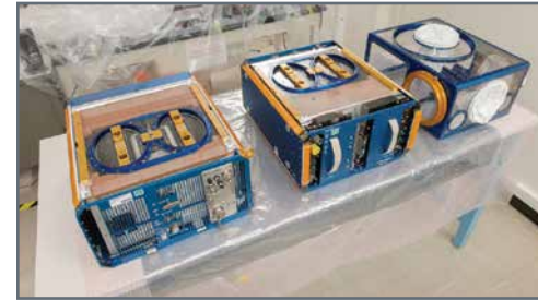
The Rodent Research Hardware System includes three modules: (left) Habitat, (center) Transporter, and (right) Animal Access Unit (NASA).
