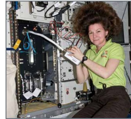
Expedition 27 Flight Engineer Cady Coleman takes electrical resistance measurements of the GHF heating units Insulation Measurement Adapter with the Multimeter volt/amp instrument during maintenance on the GHF in the Kobairo Rack (ISS027E019792).
