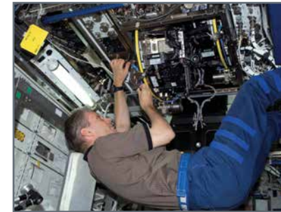
ESA astronaut Thomas Reiter installing the EMCS into EXPRESS Rack 3A (ISS013E66810).
