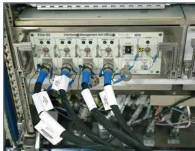
Elite S2 Interface Management Unit (ISIS Drawer) integrated in EXPRESS Rack (ISS033011716).
