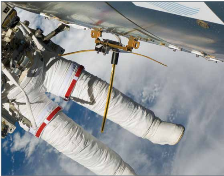
VIS Antenna shown installed on the external surface of the Columbus module (S129E007770).
