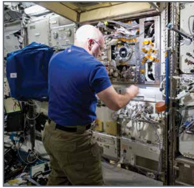
MSPR-2 ELF set up by astronaut Scott Kelly in the JEM Pressurized Module (ISS046E018682).
