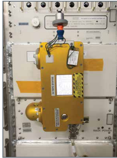
The bronze box is the IV-TEPC radiation monitor after it was located to JEM1 F3 (ISS043E241659).
