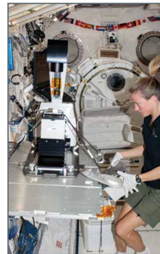
NASA astronaut Karen Nyberg works to setup the MSPR fluorescence microscope in the Kibo laboratory of the ISS during ISS Expedition 36 (ISS036E020949).
