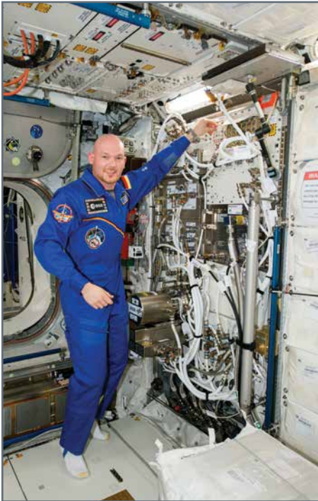
ISS crewmember Alex Gerst during installation completion of the EML inside the EDR in the Columbus module. (ISS041E107734).
