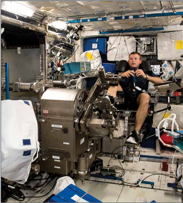
ISS crewmember Andreas Mogensen setting up the ESA MARES rack and its ankle mechanism assembly in the Columbus module. PEMS is located to the right (ISS044E101255).
