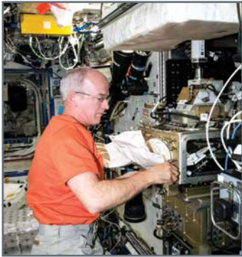
Expedition 47 ISS crewmember Jeff Williams configuring the Light Microscopy Module (LMM) for Microchannel Diffusion investigation (ISS047E066551).
