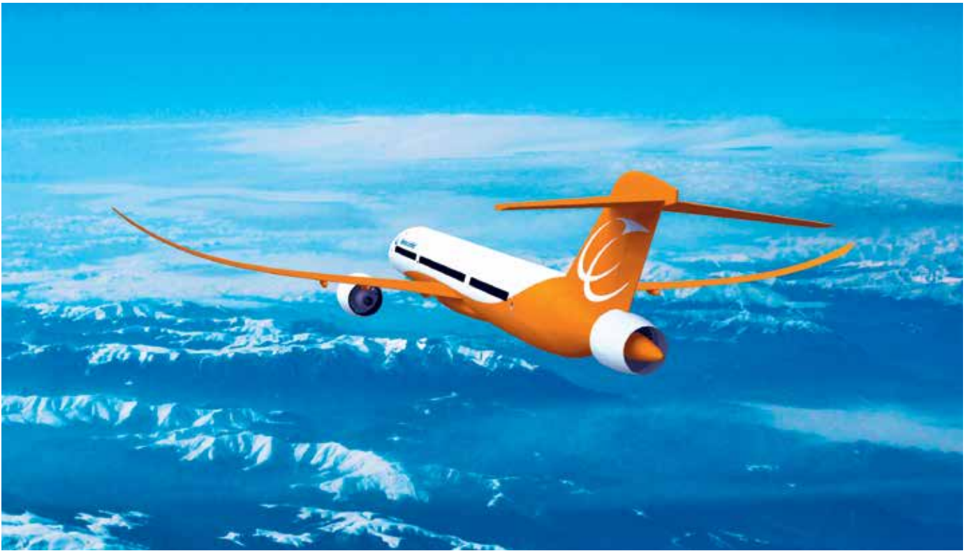
The Bauhaus Luftfahrt think tank, of which MTU is a member, is working on integrating hybrid-electric propulsion systems: in this concept study, an electrically driven propulsor is installed aft of the fuselage to facilitate wake-filling and reduce effective drag, thereby reducing the required propulsive power demand.
