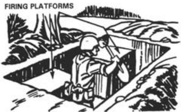
Figure 6-69. Digging T-Shaped Position.
