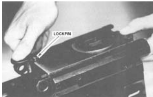
Figure 5-12. Lifting the Locking Pin.
