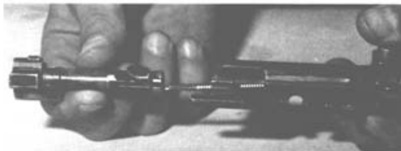
Step 2. Removing the Bolt From the Slide.
