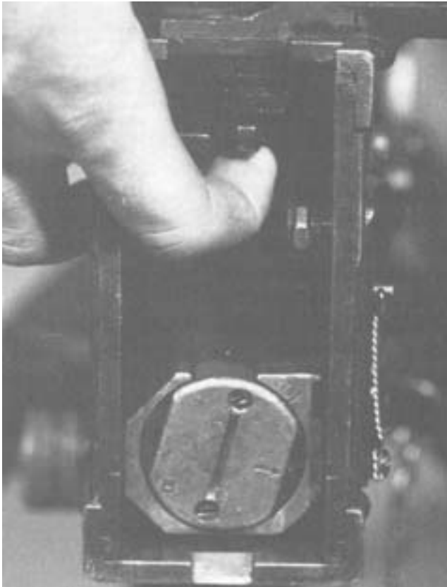
Figure 4-55. Depressing the Trigger.
