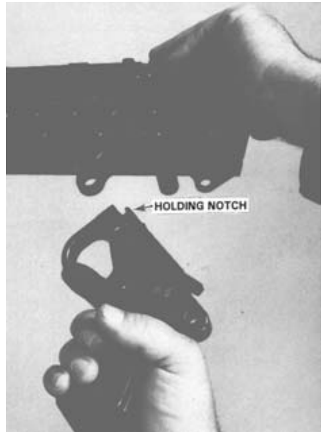
Figure 3-11. Replacing the Trigger Housing Group.
