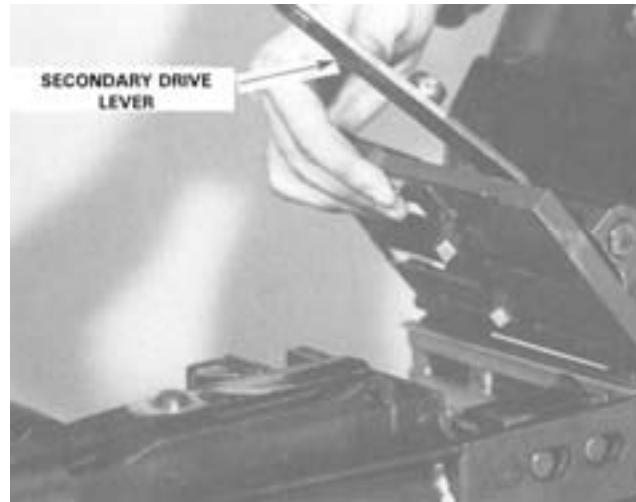
Figure 5-9. Removing the Secondary Drive Lever.
