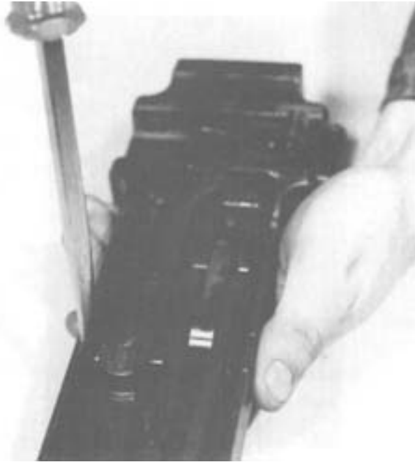
Figure 4-48. Snapping the Belt Feed Lever Lug to Seat the Shoulder Headless Pin.
