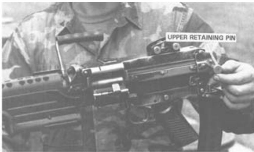
Step 1. Rotating the Buttstock Down.
