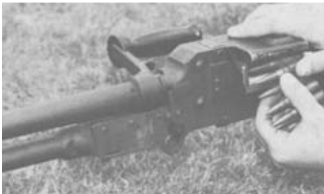
Figure 3-59. Loading, Cover Closed.
