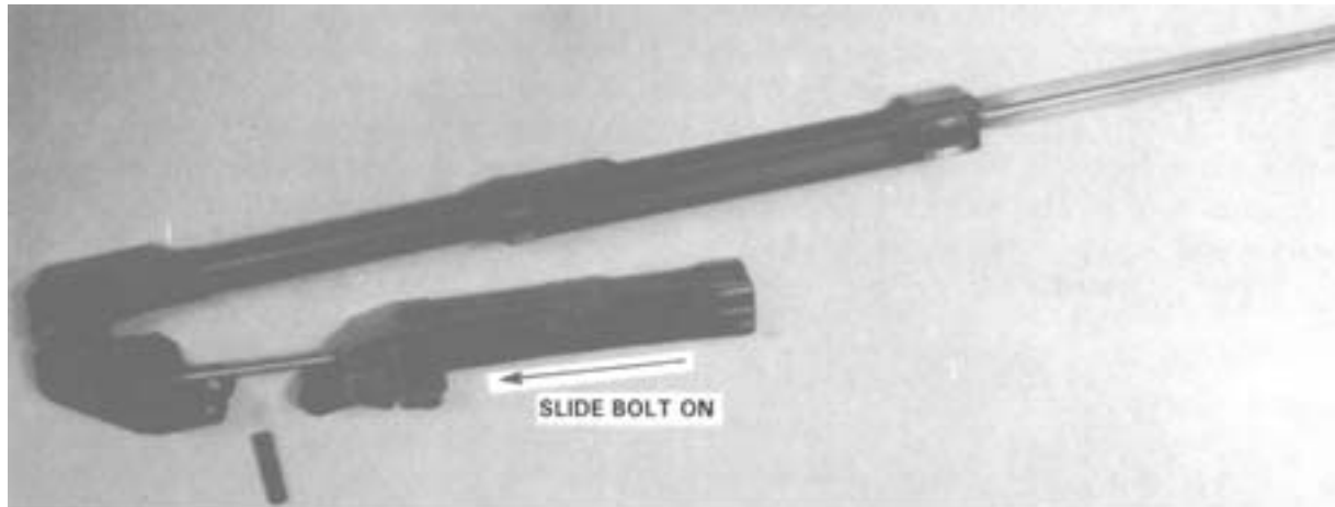
Step 1. Sliding the Bolt Over Firing Pin.
