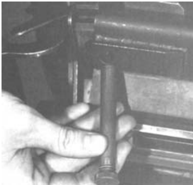
Figure 5-7. Removing the Bolt and Backplate Pin.
