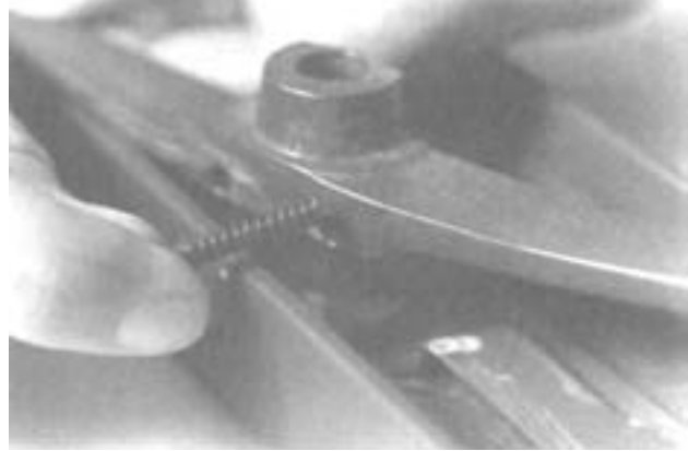
Figure 4-39. Removing the Shoulder Headless Pin and Spring.
