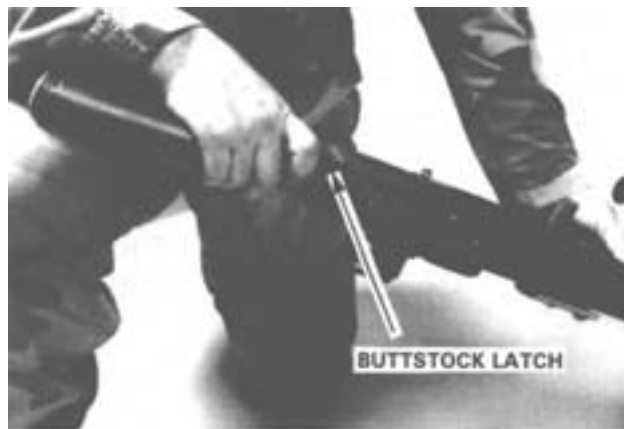
Step 1. Depressing the Buttstock Latch.
