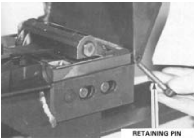
Figure 5-10. Removing the Feed Tray Cover Retaining Pin.
