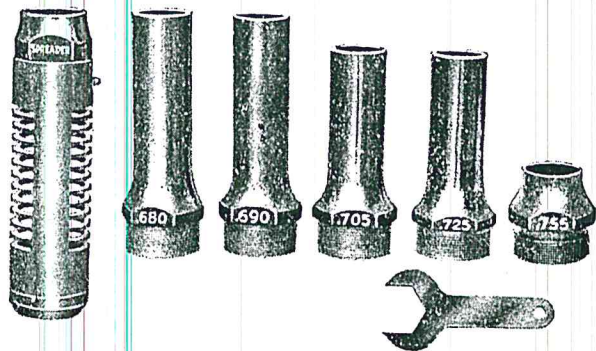
Cutts Comp for shotguns, with all 12 gauge tubes. Left to right: Comp with Spreader Tube; No. 680 or Long Range No. 2; No. 690 or Long Range No. 3; No. 705 Full Choke; No. 725 Modified Choke; No. 755 General Purpose Tube. These tubes for 12 ga. ONLY. All other gauges, Spreader, Modified and Full Choke.
