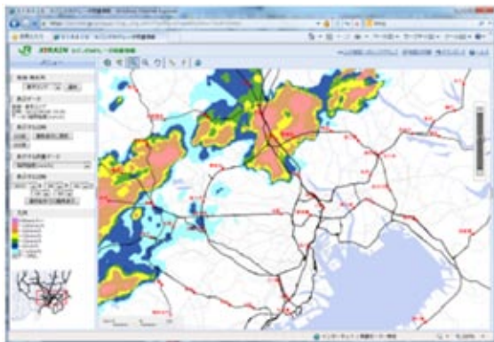
Utilization of areal precipitation information from weather radars in decision making for train operations
