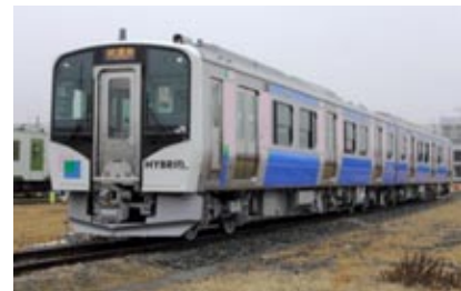
HB-E210 series: Diesel-powered, electric-motor-driven hybrid railcars
