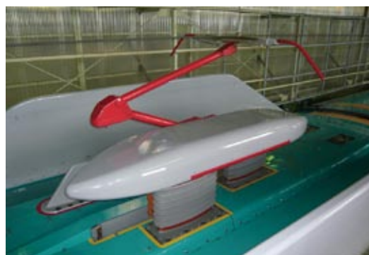
E5 Series trains have low-noise pantographs
