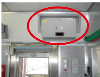
Automatic train protection radio transmission device
