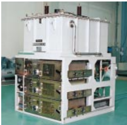
50 kW級半導体高圧パルス電源 50 kW-class, all-solid-state pulsed power generator
