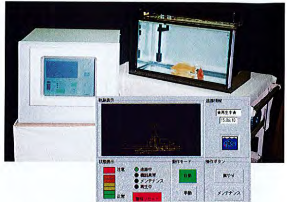
上水原水毒物検出支援装置 Toxicity detection support systems for raw water
