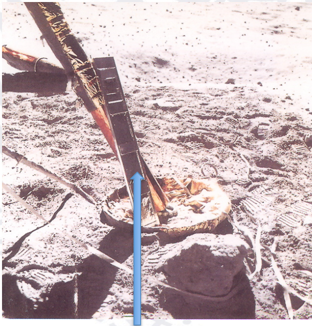
The DIAS-Berkeley detectors resting against the lunar module leg on the lunar surface
