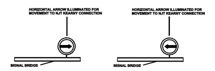
White directional indicator arrows in service for westward movements on No. 2 and No. 3 tracks at MP 6.3 and home signals at Swift. When route at Swift is lined for diverging movement to NJT Kearny Connection from No. 2 track to No. 6 track or from No. 3 track to No. 5 track, directional indicator arrows will display at **both** Swift and MP 6.3.
