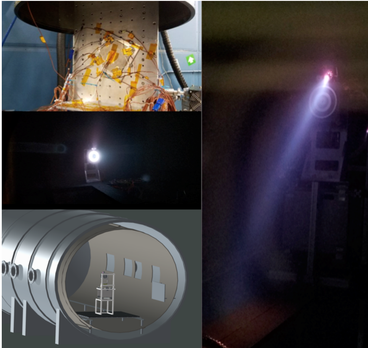
Figure 11. Belljars for thermal gasket testing (top), the 6x10 chamber for cathode testing (right), and the 10x20 chamber for 1.5kW thruster operation (center, lower).
