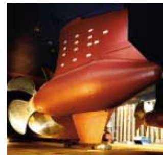
2 x 20 MW Azipod® units installed on Radiance of the Seas
