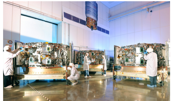
The Cygnus Service Module incorporates systems from Orbital ATK's flight proven LEOStar and GEOStar satellite product lines
