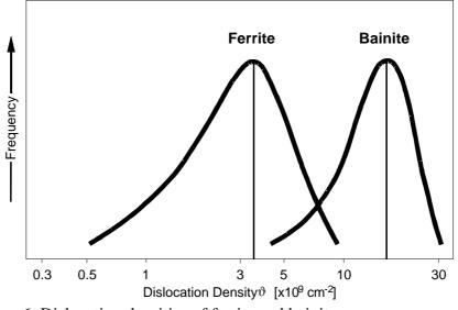
Figure 6: Dislocation densities of ferrite and bainite
