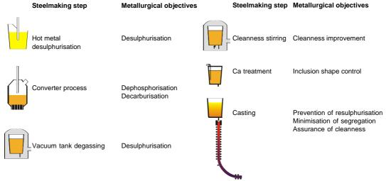
Figure 23: Production steps of steels with high cleanness requirements for sour service
