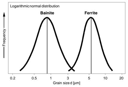
Figure 5: Grain sizes of ferrite and bainite
