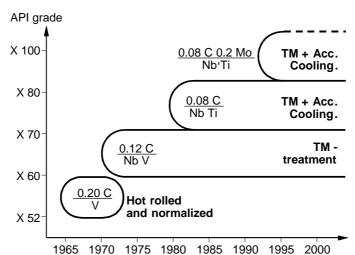
Figure 1: Development of High Strength Steels
