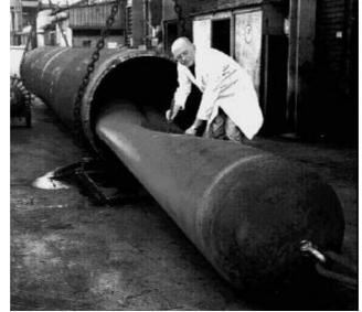
Figure 21: Photograph showing buckled linepipe section
