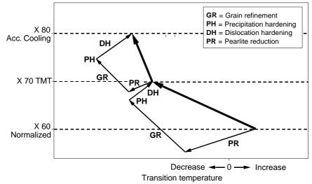
Figure 2: Microstructural effects for enhancing strength and toughness properties
