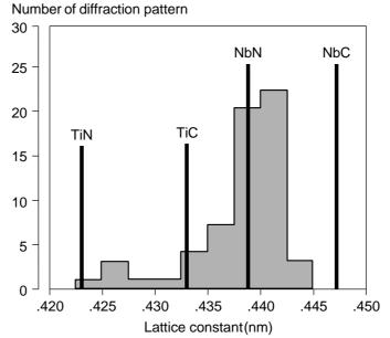
Figure 10: Distribution of lattice constants of carbonitrides in MnNb-steels Number of diffraction pattern
