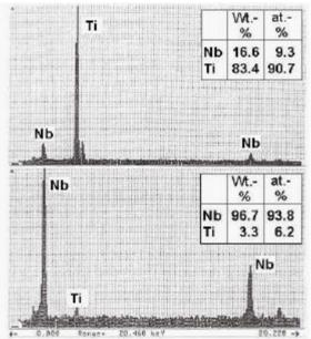
Figure 12: EDX-analysis of carbonitride precipitations
