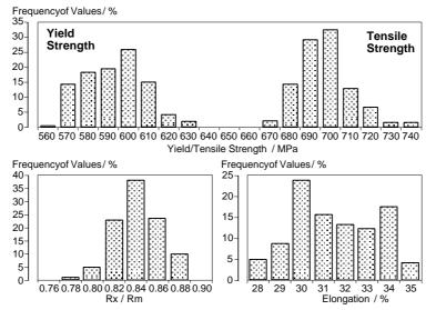
Figure 16: Distribution of mechanical properties of 48"diam. X80 linepipe with 15.1 mm wt
