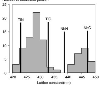
Figure 11: Distribution of lattice constants of carbonitrides in MnNbTi-steels
