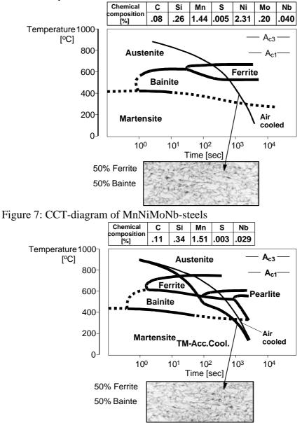
Figure 8: CCT-diagram of accelerated cooled MnNb-steels
