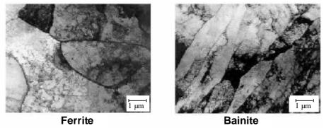
Figure 4: TEM microstructures of ferrite and bainite
