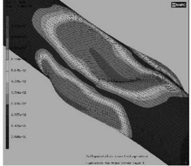
Figure 22: Simulation of collapse behaviour with FEA
