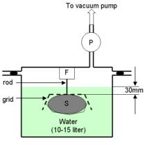
Airtight tank (approved for the pressure) connected to a vacuum pump P: vacuum pressure transducer (~10-1000mbar) F: force transducer (~50N) S: swim suit
