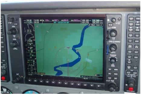
Many instrument-capable general aviation aircraft have GPS receivers and moving map displays.
