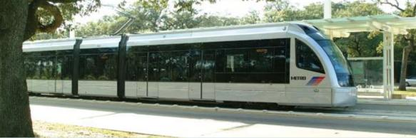
Bi-directional six-axle, low floor articulated light rail vehicle constructed of low alloy high tensile (LAHT) steel and composite materials with concealed couplers.
