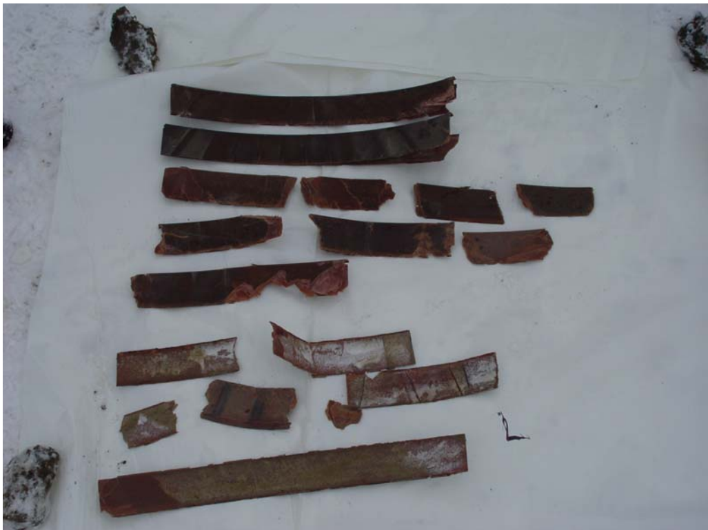
Attachment 10: All loose ice impact panels of the LH engine
