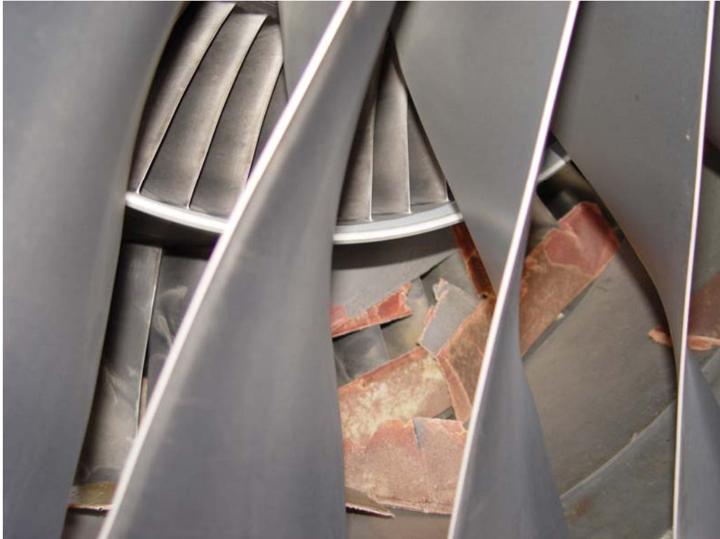
Attachment 9: Loose ice impact panels in the LH engine intake
