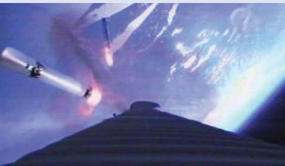
“Rocket Cam” image of Solid Rocket Booster jettison as the Atlas rocket flies away from Earth.
