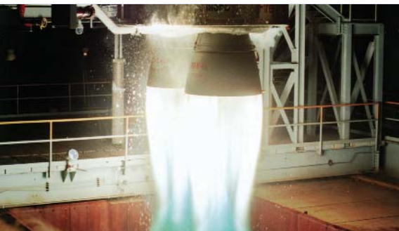
The powerful RD-180 engine firing during a test.
