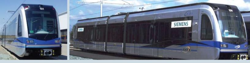
Bi-directional, six-axle, low floor articulated light rail vehicle constructed of low alloy high tensile (LAHT) steel and composite materials.
