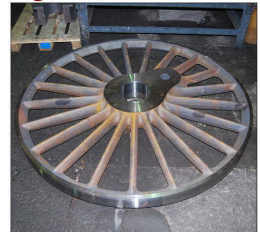
▲ The first driving wheel that has been cast for The Unknown Warrior has now been machined at the Boro Foundry in the West Midlands. LMS-Patriot Project
