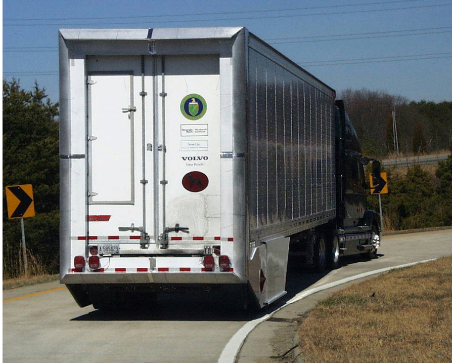
Fig 21. Coanda blowing of flat backed trucks yields 11% to 12 % fuel saving. The technology is owned by Georgia Tech Research Institute. Download report from Georgia Tech at: http://newfluidtechnology.com.au/GTRI.pdf
