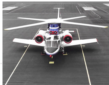
There is no mechanism present for cyclic and collective pitch control on this later version.
