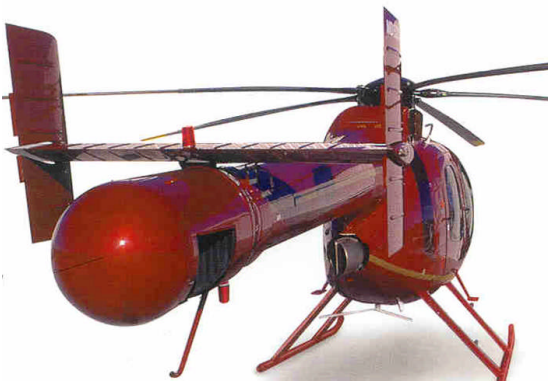
Fig 28. No Tail Rotor helicopter (NOTAR): Coanda jet lowers pressure over boom for directional control.
