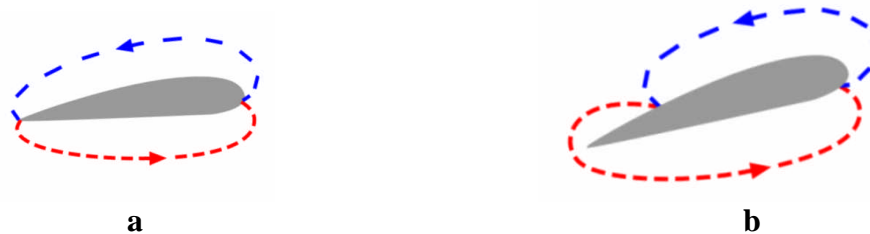
Fig 16. These are strictly schematic diagrams. a , stagnation points in normal unstalled positions. For b ; the rear stagnation point shifts upstream resulting in stall.
