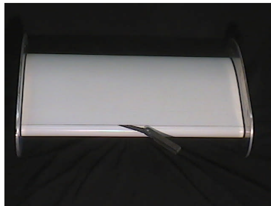
Fig 30. New Fluid Technology Coanda wind turbine blade section. :Setting slot height.
