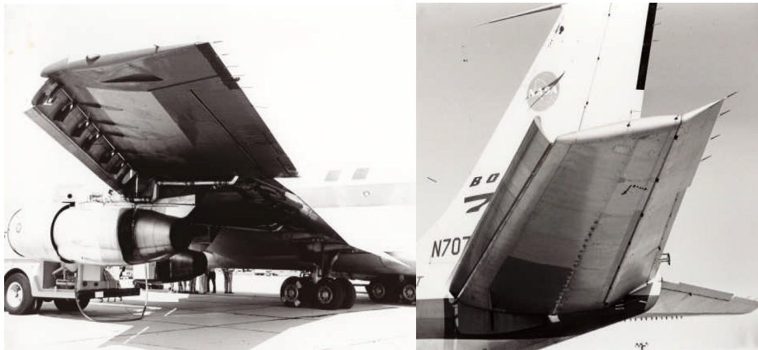
Fig 18. Boeing 387-80 prototype of the 707 airliner on the ramp at NASA Wallops Station, Virginia, in June 1964 . The "Dash 80" had been modified for very slow flight using wing flaps blown by Coanda Effect. Primary air for blowing the flaps came from compressor bleed of the Number One and Number Four engines. Aircraft could fly as slow as 70 knots. Caption by G. Harry Stine. (70 knots = 80.6 mph = 129.85 kph which is about half its normal takeoff speed).
