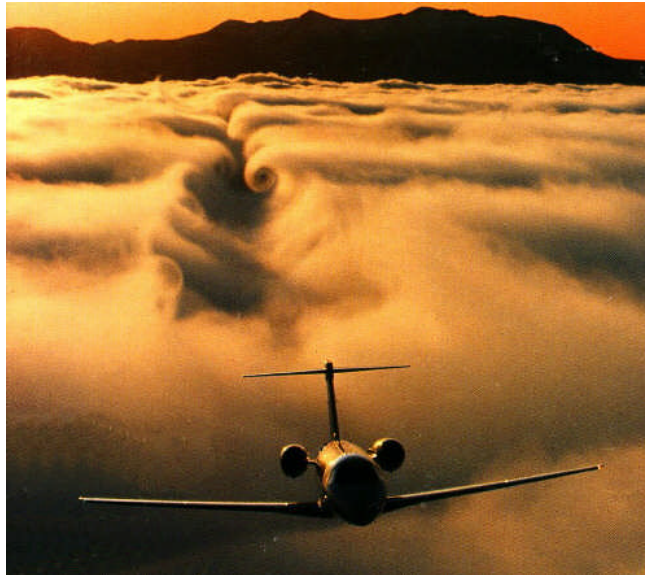
Fig 8. Cloud pattern merely makes visible the trailing tip vortices depicted schematically in Fig 7 and 9.
