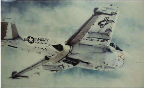
Fig 19. A 6 with bluff wing trailing edge; 1979.
