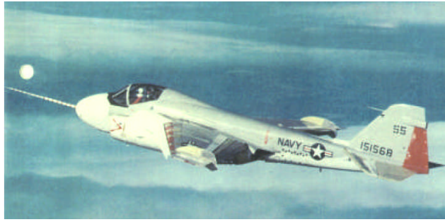
CC applied to this aircraft enabled a 75% increase in payload.
