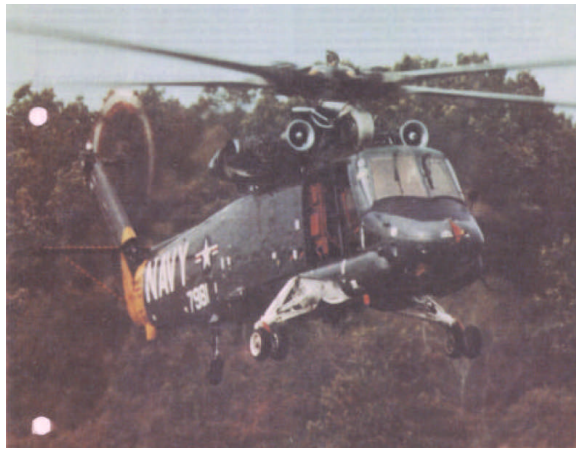
Fig 20. Navy/Kaman Aerospace, Circulation Control (CC) helicopter.
