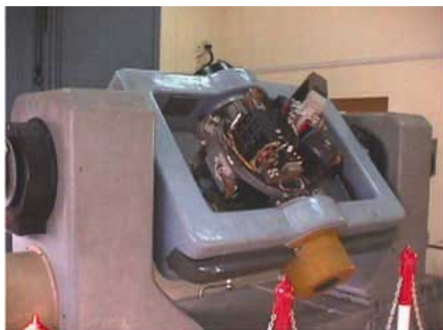
Figure 12. Angular motion simulator.
