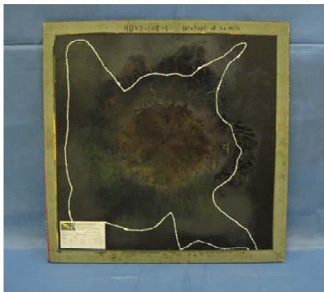
Hontek 0.020 inch thick (same as Full Blade Test)
