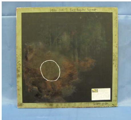
Bell Topcoat (0.005-0.007 inch thick)
