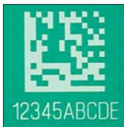
FIGURE 1. Example of ECC 200 Data Matrix code on FR-4.
