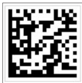
FIGURE 2. ECC 200 code marked in black ink, suitable for ceramic substrates.
