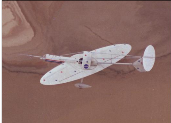
Figure 29. NASA Ames oblique wing remotely piloted vehicle (first flight 1976). Maneuvers were performed at wing angles of 0 to 45°. The long tail is noteworthy. (Photo courtesy of the NASA Dryden Flight Research Center.)
