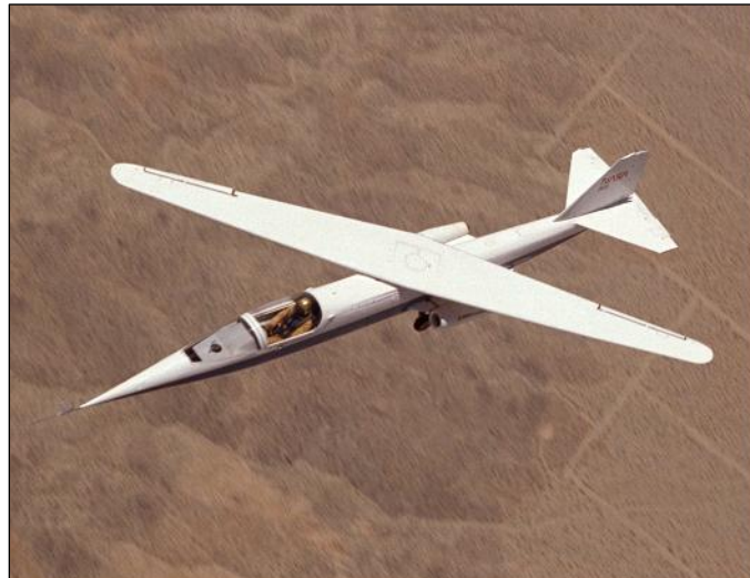
Figure 32. Ames-Dryden AD-1 oblique wing demonstrator (first flight 1979). It flew with the wing at angles from 0° up to 60° and speeds up to 150 kt. (Photo courtesy of the NASA Dryden Flight Research Center.)
