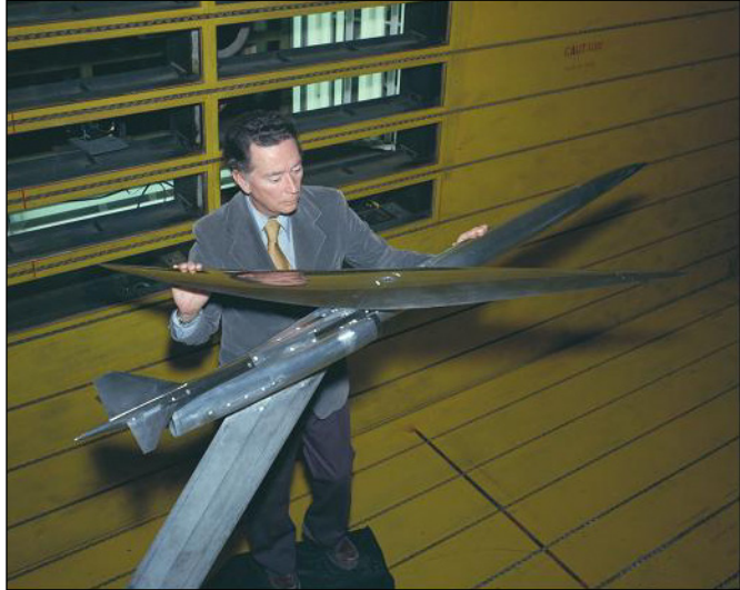
Figure 17. R.T. Jones with the oblique wing model used for the Convair wind tunnel testing. This photo shows the integrated propulsion system, as well as where the model mounted on the blade support. (Photo courtesy of the NASA Ames Research Center.)
