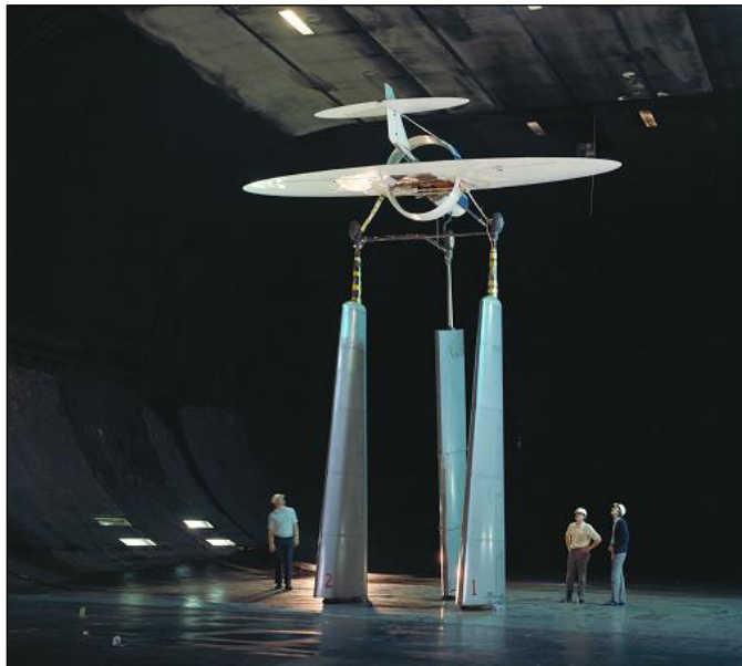
Figure 28. The Oblique Wing RPV in the NASA Ames 40 ft by 80 ft wind tunnel. (Photo courtesy of the NASA Ames Research Center.)
