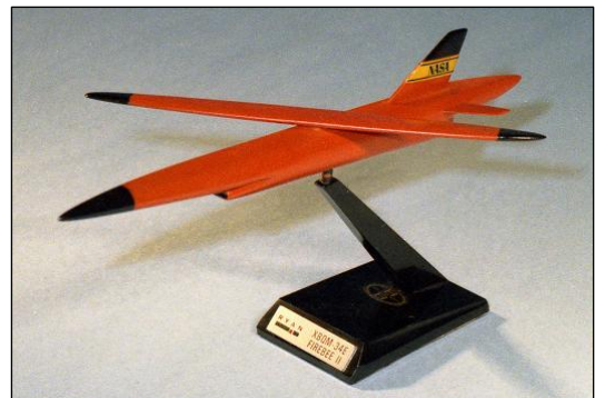
Figure 30. Model of the Oblique Wing Firebee II RPV. (Photo courtesy of the NASA Dryden Flight Research Center.)
