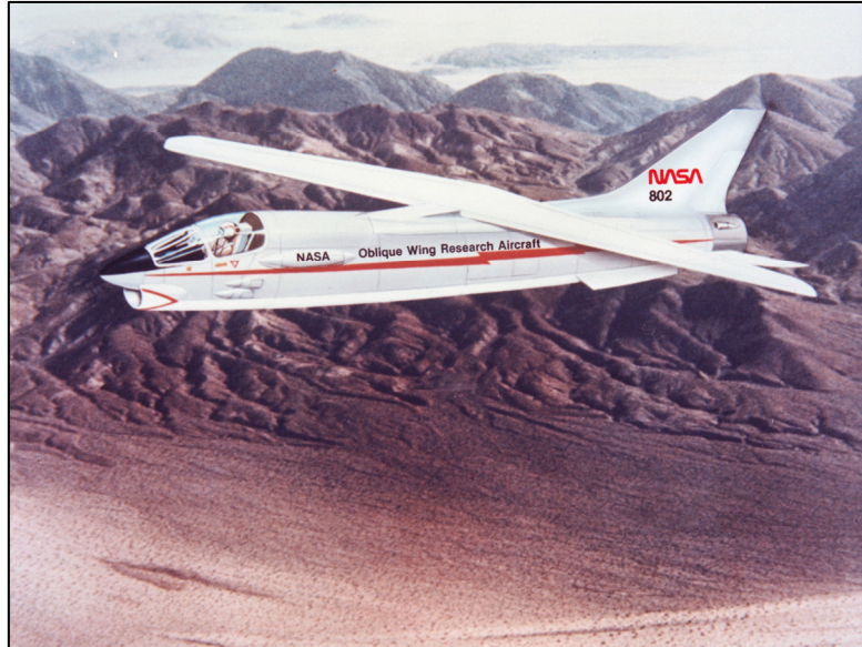
Figure 38. Proposed supersonic F-8 Oblique Wing Research Aircraft. (Graphic Courtesy of the NASA Ames Research Center.)
