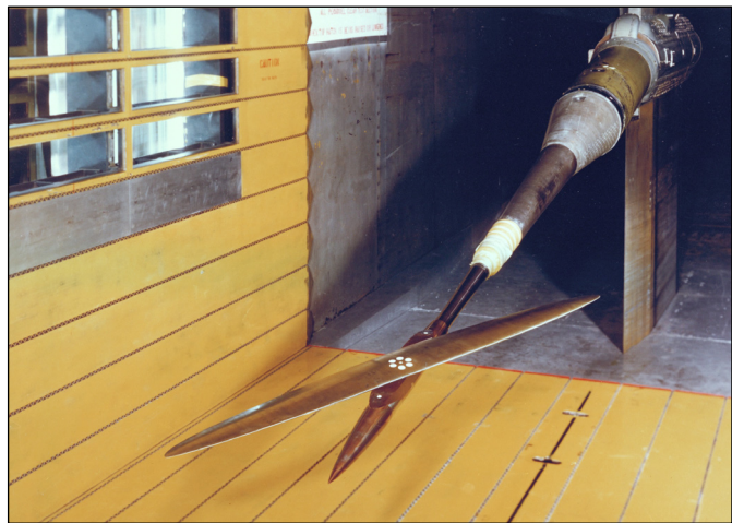
Figure 16. High aspect ratio oblique wing model in the NASA Ames wind tunnel at 60° sweep. (Photo courtesy of the NASA Dryden Flight Research Center.)
