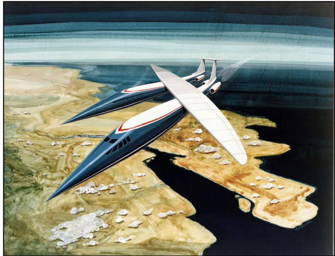
Figure 13. R.T. Jones' twin-fuselage oblique wing transonic transport. With the exception of minor changes to the wing shape, this painting is identical to Jones' patent (filed in 1971).
