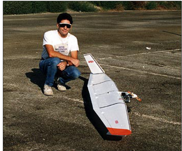
Figure 48. Steve Morris’ 10 ft OFW (first flight 1993). It flew at sweep angles of up to 65°. (Photo courtesy of Steve Morris. Used with permission.)
