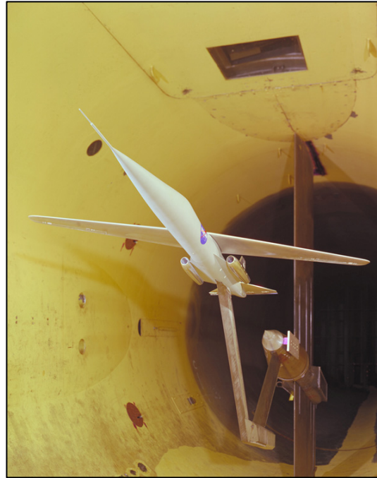
Figure 31. AD-1 one-sixth scale model in the NASA Ames pressure tunnel. (Photo courtesy of the NASA Ames Research Center.)
