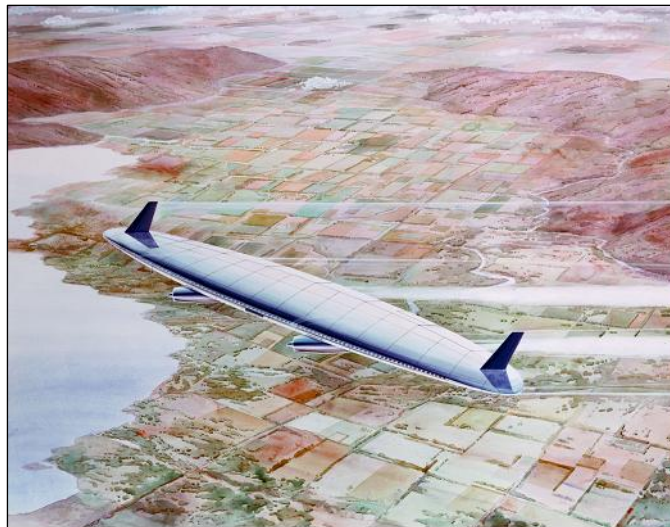
Figure 40. Artwork of Jones' OFW concept (1989). Right wing tip is forward. (Graphic courtesy of the NASA Ames Research Center.)
