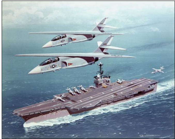
Figure 34. Rockwell concept for a Navy oblique wing aircraft, based on their VFMX fleet air defense studies. (Graphic courtesy of the NASA Dryden Flight Research Center.)
