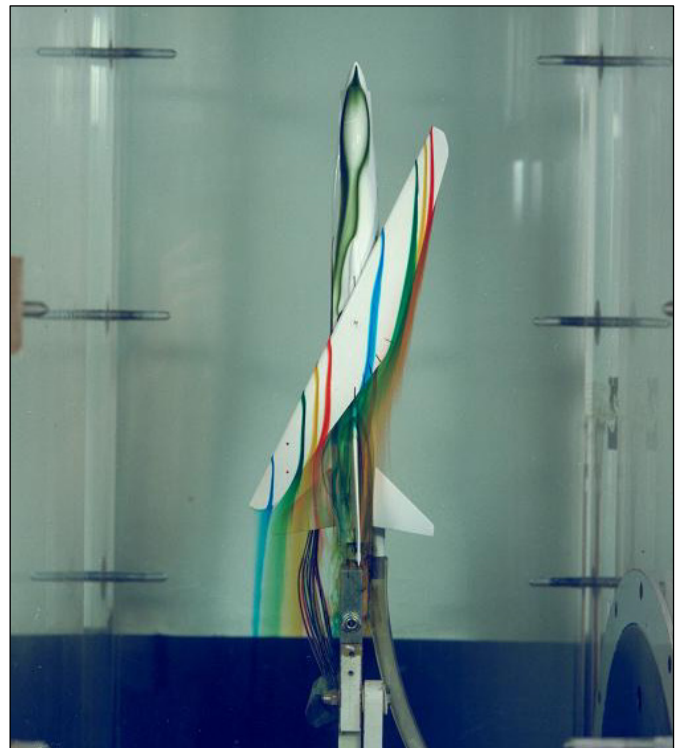
Figure 35. 1984 water tunnel test of the F-8 OWRA. (Graphic courtesy of the NASA Dryden Flight Research Center.)
