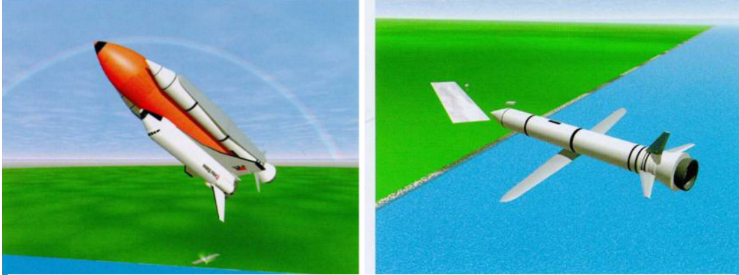
Figure 23. 1999 study of an oblique wing fly-back capability for the space shuttle booster. 46
