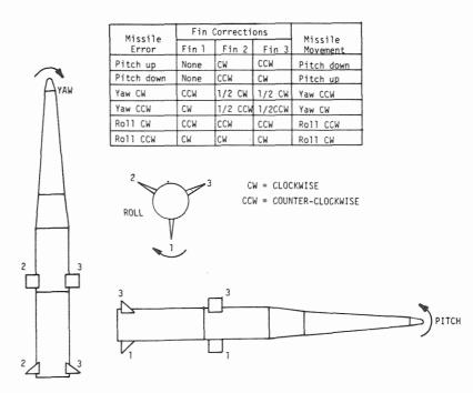
Figure 2-10. Missile Response to Attitude Errors
