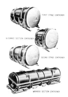
Figure 1-13. Missile Section Shipping and Storage Containers
