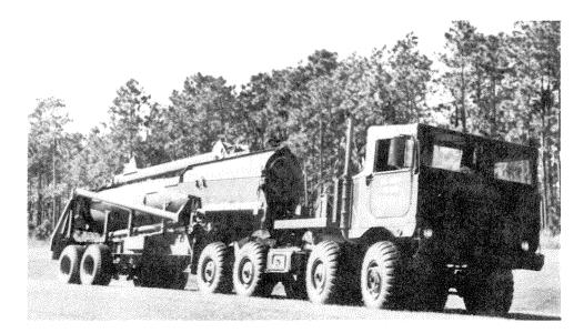
Figure 1-4. Tractor with Erector-Launcher
