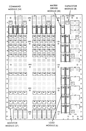
Figure 4-9. Adapter Register Board 32A2A5 Module Locations
