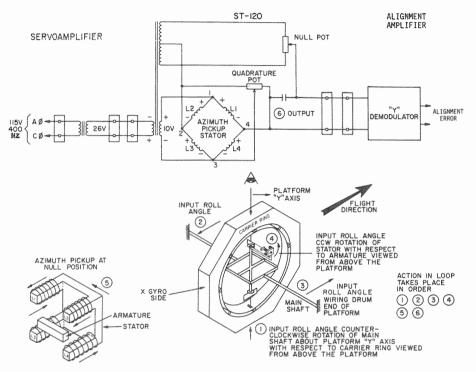
Figure 2-26. Azimuth Pickoff Operation
