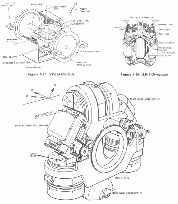
Figure 2-19. ST-120 Accelerometer Orientation and Subassembly Location
