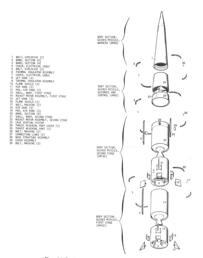
Figure 2-1. Pershing Missile Aero and Structural Components
