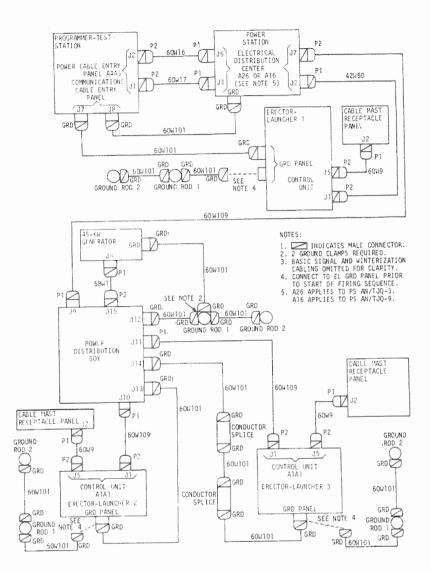
Figure 9-2. QRA Tactical Site, Standby Power Distribution
