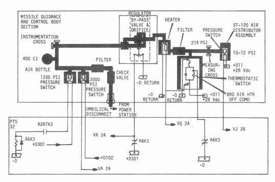
Figure 2-30. Air System Functional Diagram
