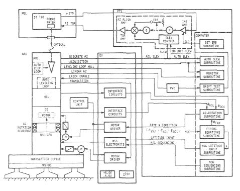
Figure 11-4. ARS Block Diagram
