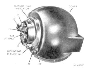
Figure 2-15. ST-120 Inertial System
