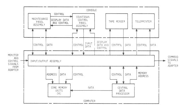
Figure 4-5. Computer Block Diagram
