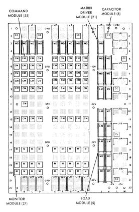
Figure 4-8. Adapter Register Board 32A2A4 Module Locations
