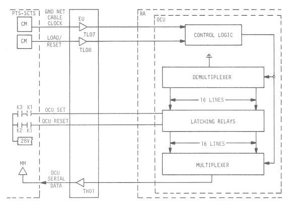
Figure 11-7. Offset Correction Unit Block Diagram
