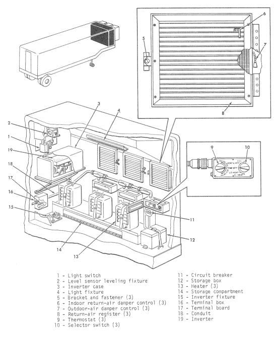
Figure 10-9. Interior View of Forward Storage Compartment
