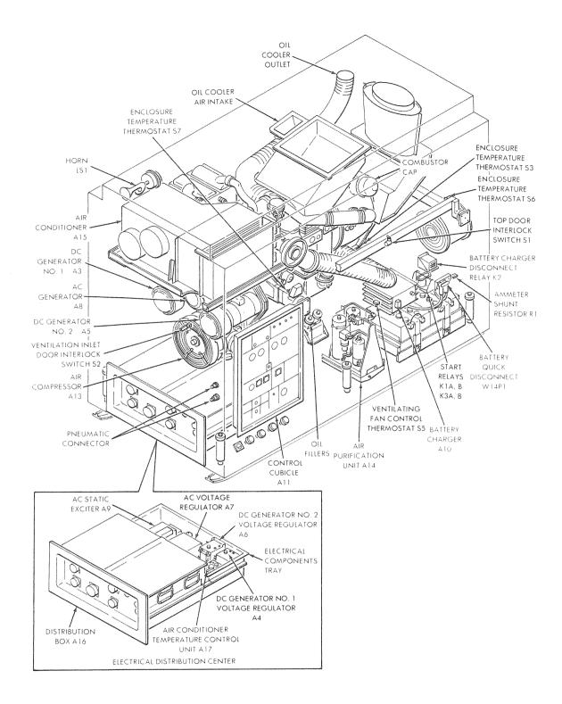
Figure 5-2. PS Three Quarter Front Internal View
