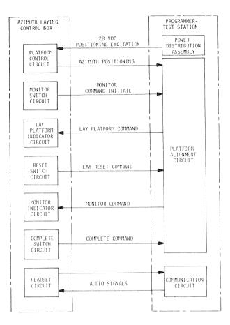
Figure 6-6. Azimuth Laying Control Box Signal Flow Diagram
