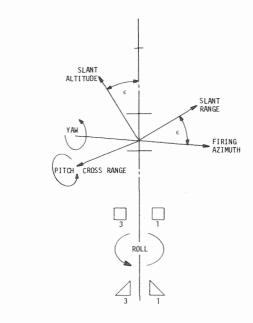
Figure 2-11. Missile Coordinate System
