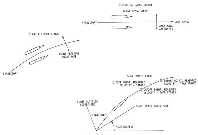
Figure 2-8. Missile Guidance Coordinates and Errors
