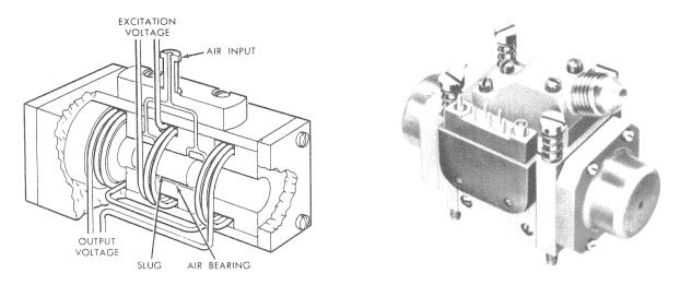
Figure 2-24. Air Bearing Pendulum
