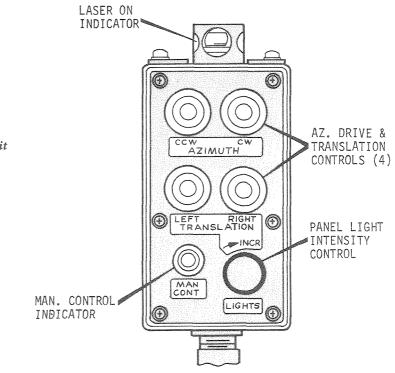
Figure 11-11. Manual Control Unit
