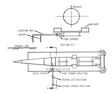
Figure 11-12. Tripod Emplacement Device
