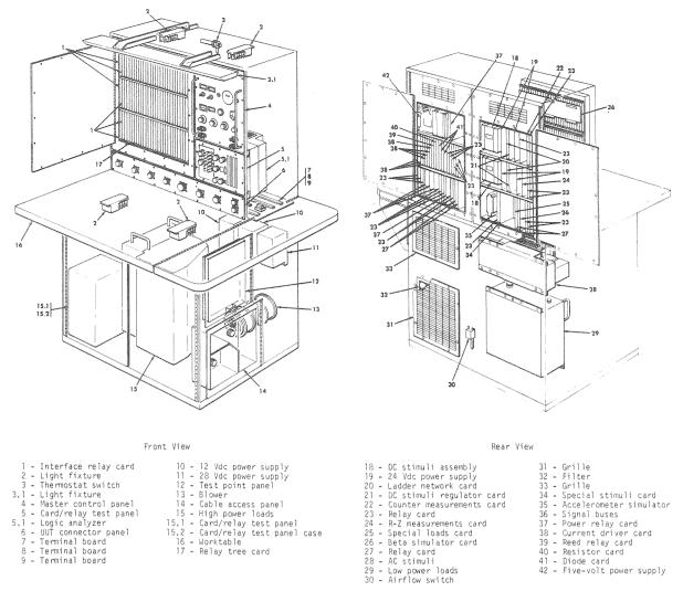
Figure 10-3. Assembly Tester
