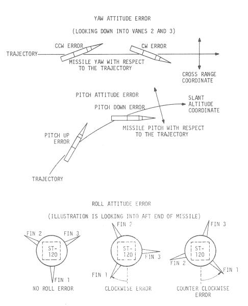
Figure 2-9. Missile Attitude Errors
