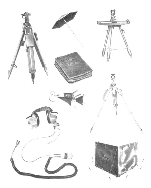
Figure 1-6. Azimuth Laying Set
