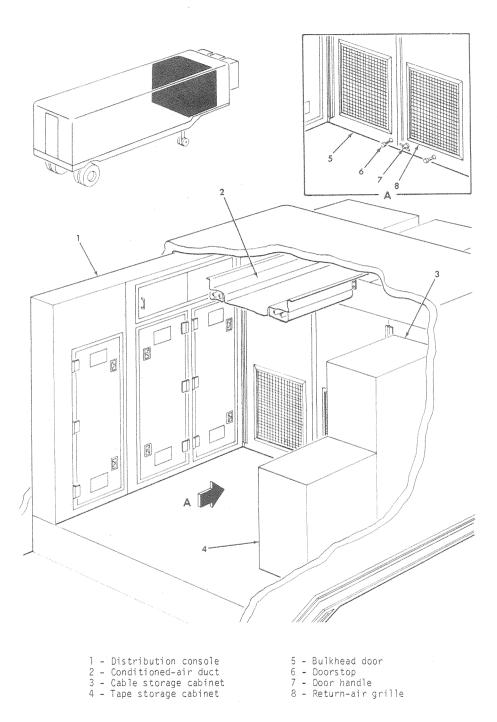
Figure 10-8. Exterior View of Forward Storage Compartment
