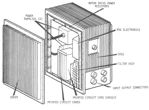
Figure 11-8. Electronics Unit
