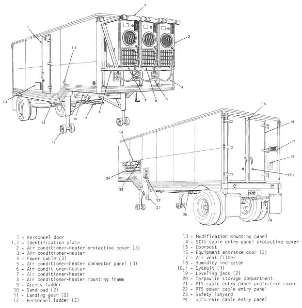
Figure 10-1. System Components Test Station Exterior View
