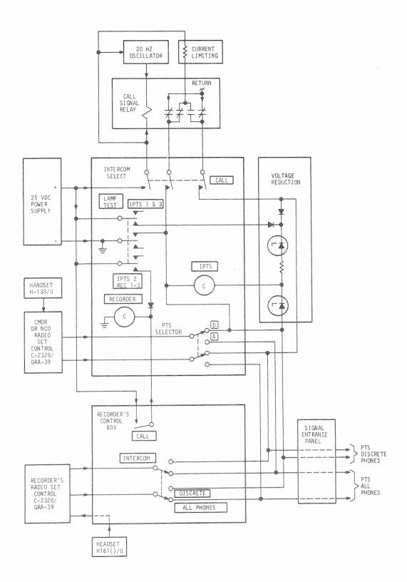
Figure 7-2. BCC/PTS Typical Intercommunications Schematic
