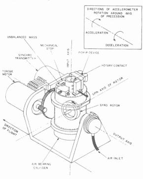
Figure 2-23. Integrating Accelerometer
