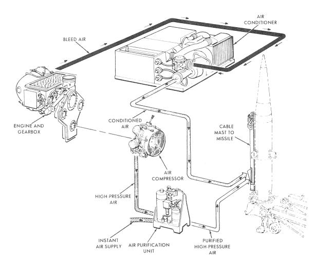
Figure 5-5. Air System Flow Diagram
