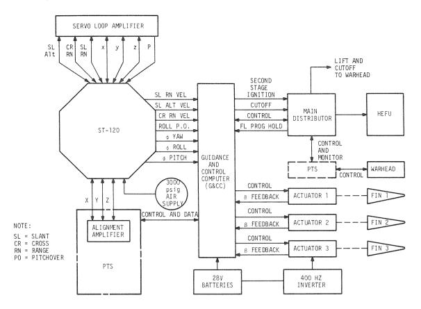
Figure 2-7. Guidance and Control System Functional Schematic
