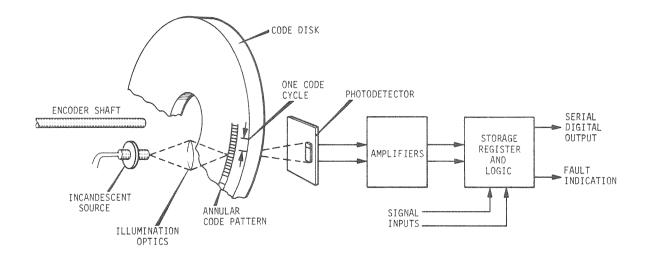
Figure 11-6. Digital Encoder Functional Schematic
