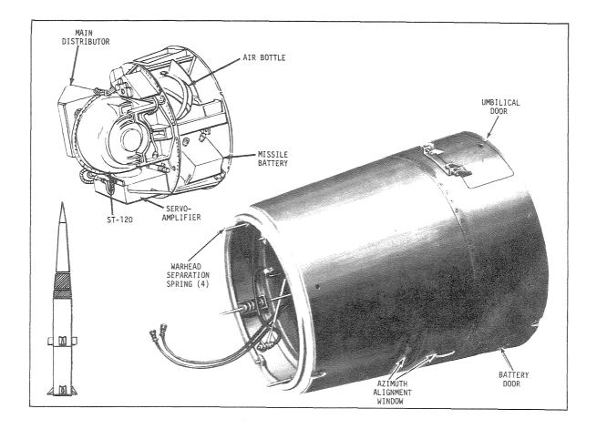
Figure 2-6. Guidance and Control Section
