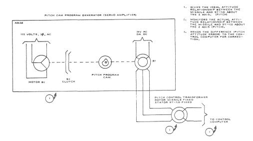
Figure 2-28. Pitch Cam Program Generator
