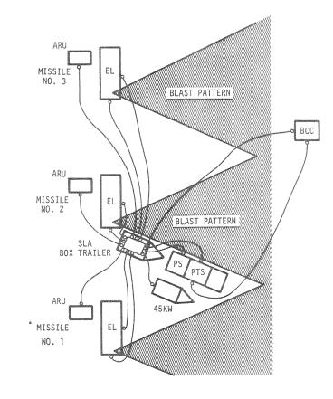
Figure 11-14. SLA Tactical Site Layout Configuration
