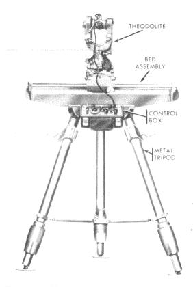
Figure 6-2. Horizontal or Vertical Laying Theodolite with Control Box
