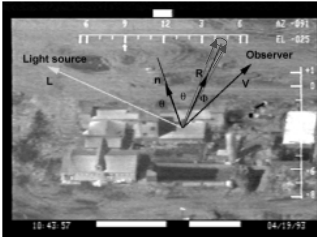
Fig. 5. An illustration of the geometrical reflection model.
