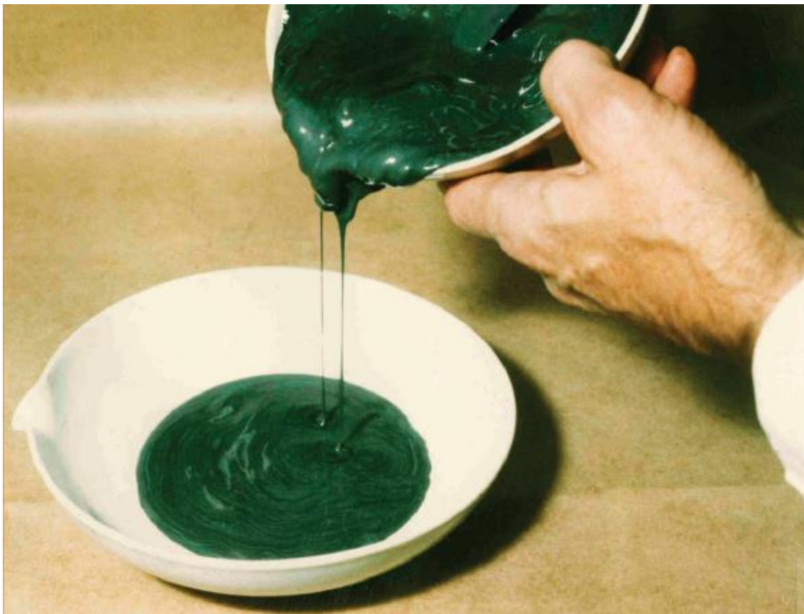
Figure 2.3: Shows the liquid quick clay when stirred or overloaded (Issler et al., 2012).
