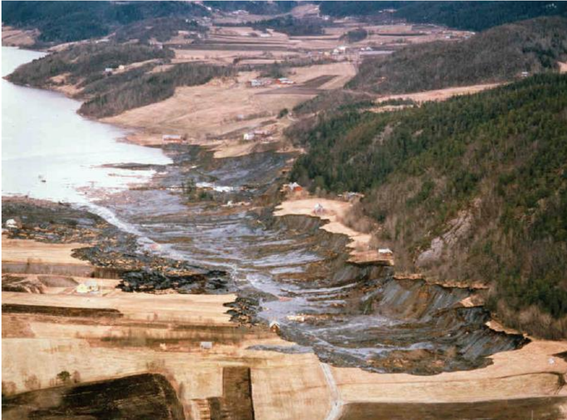
Figure 2.1: Shows the landslide crater after the Rissa landslide. The length of the crater measures 1,5 km (NVE, 2006a).
