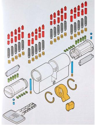
120 parts used in a DOM ix double profile cylinder
