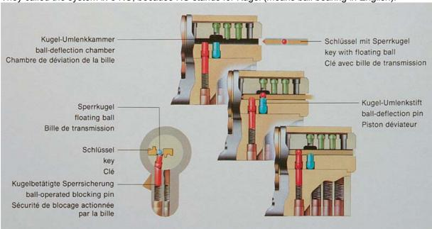
Working of the floating ball in the key in three phases
