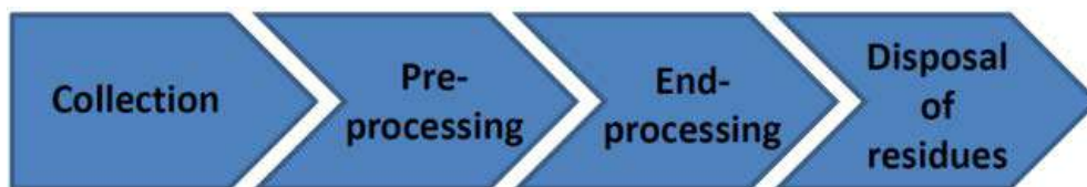
Figure 5-2: Generic recycling chain for end-of-life EEE
