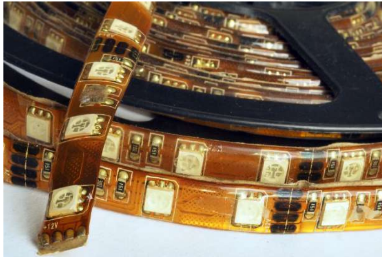
Figure 5-1: Flexible LED-stripe (Light Emitting Diodes) containing internal wiring and insulation based on flexible polymers
