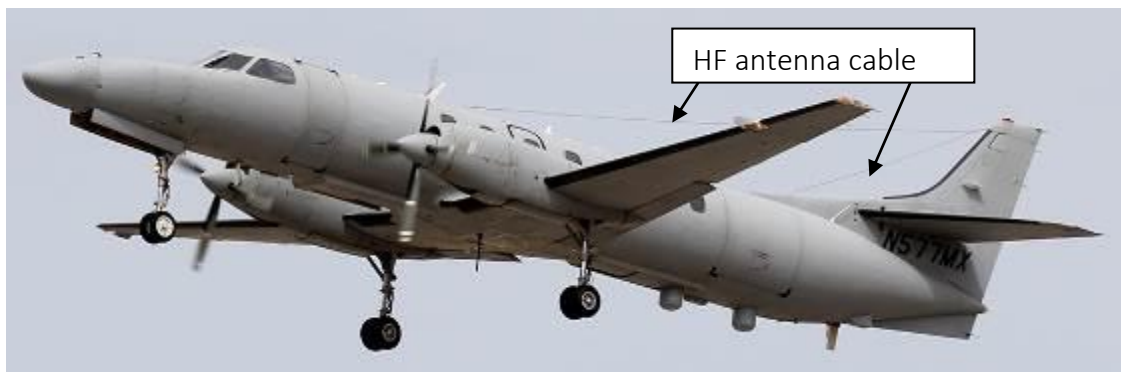
Figure 25: Position of the HF cable on the aircraft
