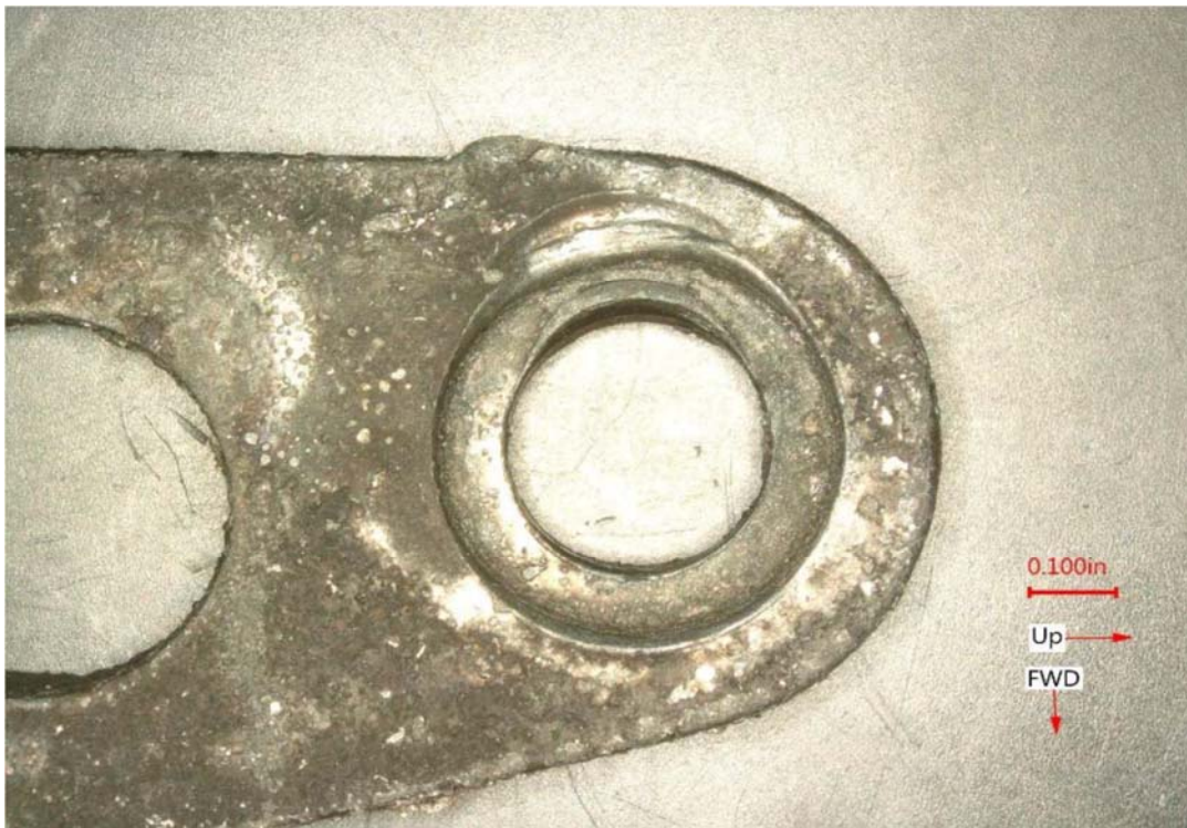
Figure 23. L1 cabin crew seat pan hole elongated [Source: NTSB]
