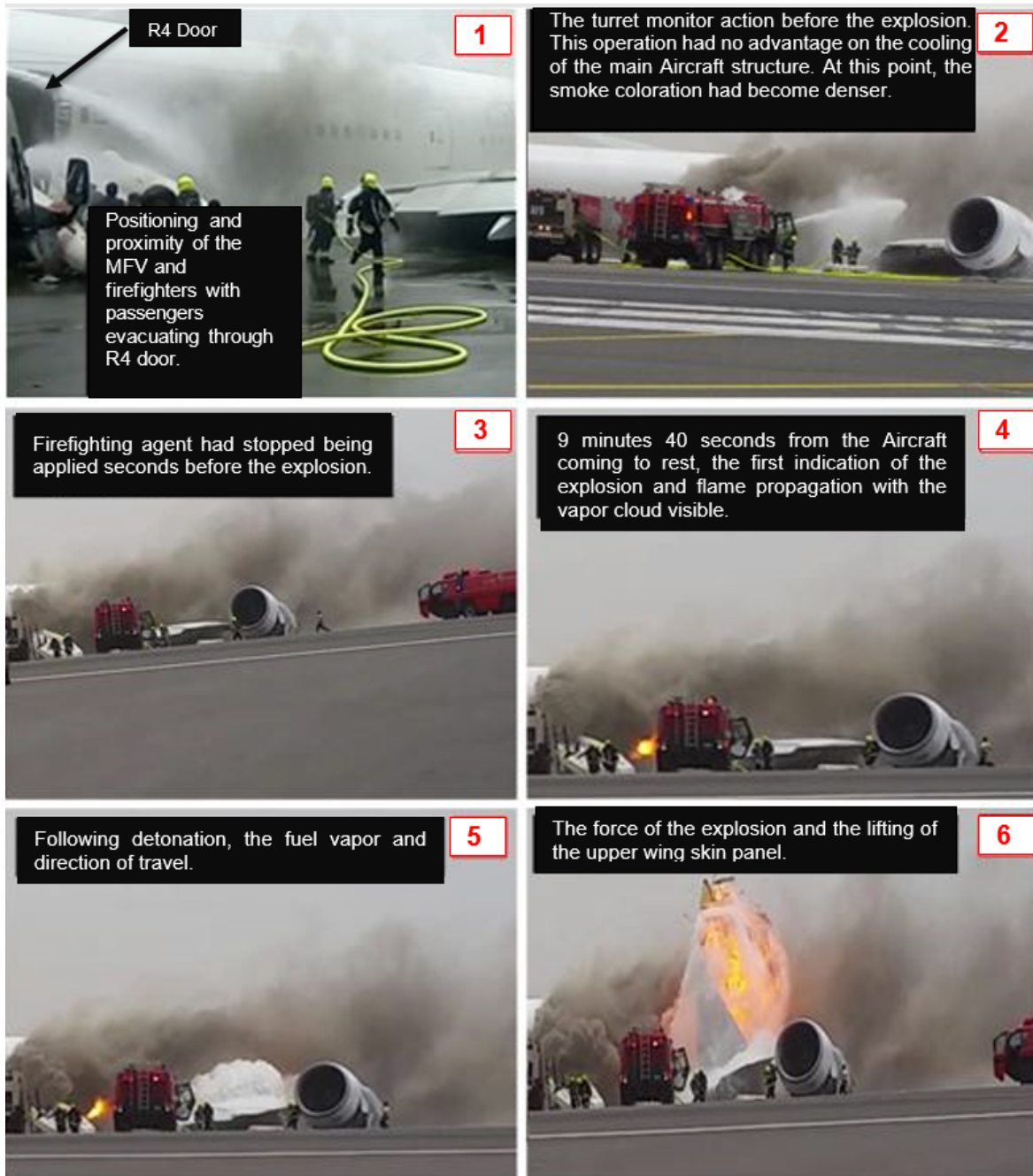
Figure 17. Center wing fuel tank explosion
