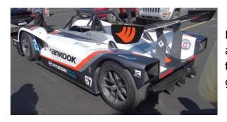
Rhys Millen returns in 2016 in the '16 e0 PP100 for a time of 8:57.118. There are four motors ganged together to create one to drive the rear, and three ganged together to create one to drive the front.
