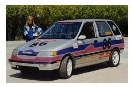
1994 was the first year for an "Electric" Class at the Hill Climb which brought out four competitors. The winner, beating the others by six to nine minutes, was Katy Endicott at 15:44.71. This converted 1991 Honda used 25ea 12V Sealed Lead Acid Batteries, powering a 65kW Brushless DC Motor with Regenerative Braking.
