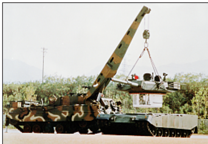
K1 armoured recovery vehicle with crane traversed to front and stabiliser/ dozer blade lowered and lifting complete K1 MBT turret
