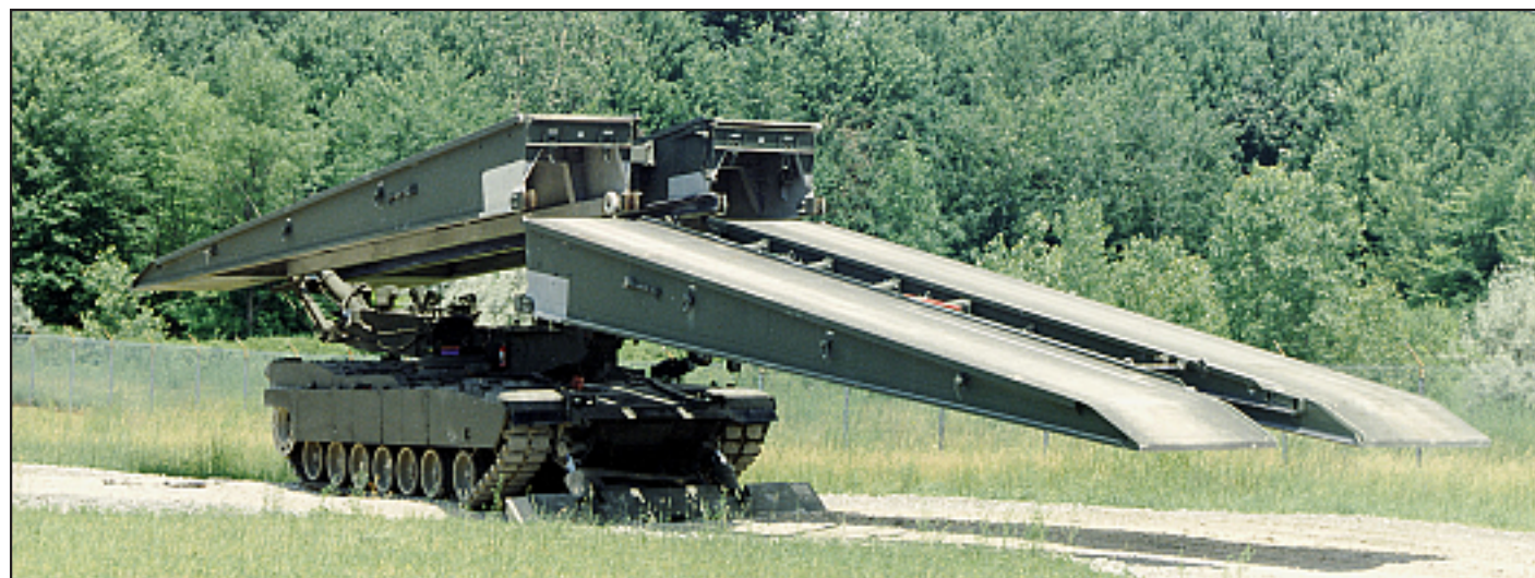
Heavy Assault Bridge with 26 m bridge being extended over front of vehicle
