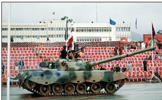
NORINCO Type 85-II AP MBT in service with Pakistan and showing roof mounted 12.7 mm machine gun 1403755
