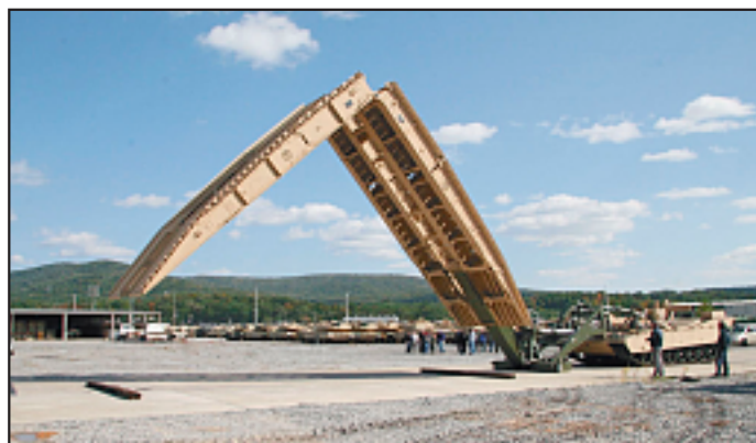
Original Joint Assault Bridge laying its scissors bridge over the front of the modified M1 Abrams series MBT hull (US Army) 1340084
