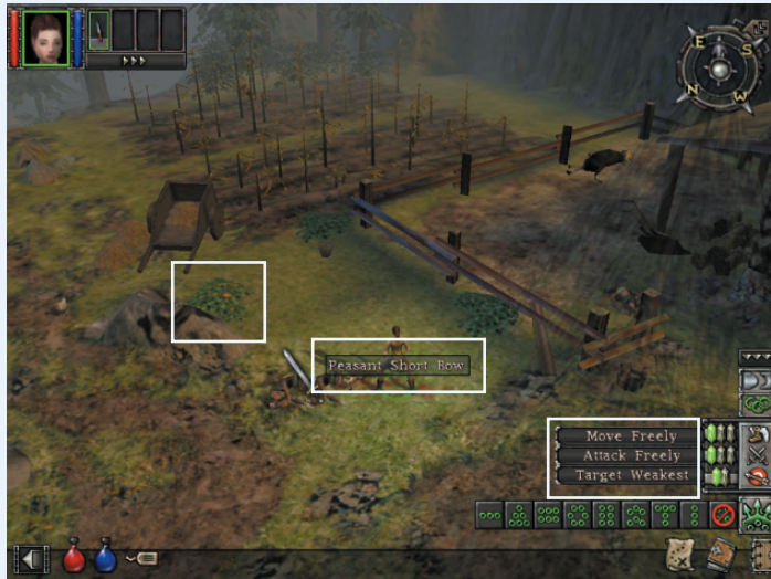
Figure 7 - Notice the heavy blurring in the multisampling example as compared to FAA-16x. While only a few examples have been highlighted, the blurring is visible across the entire scene (scene from Microsoft® Dungeon Siege).
