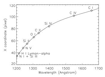
**Fig. 2.** Plot of the wavelength calibration. The squares show the position of each identified emission feature as a function of wavelength. The solid line shows the fit by a third-degree polynomial.
