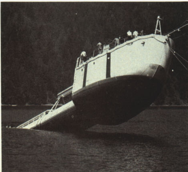
Below: The tube portion of FLIP is flooded with seawater to achieve its upright position. Left: FLIP, ready to begin studies.
