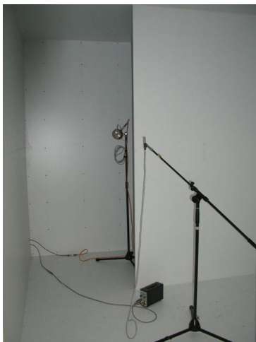
Figure 2: Additional panels can be mounted inside the Bell Labs box to study the effects of sound diffraction.
