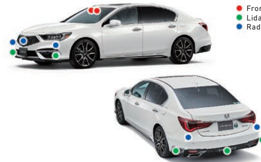
Layout of sensors of the Honda Sensing Elite
