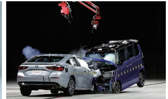
Omni-directional crash test facility
