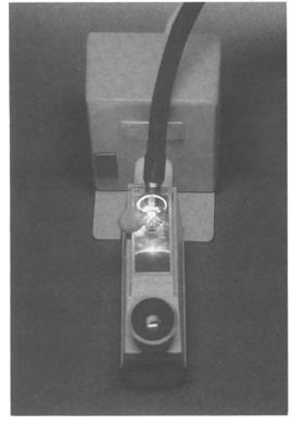
Fig. 2. Fibre optic light source directed on to the stone under test.
