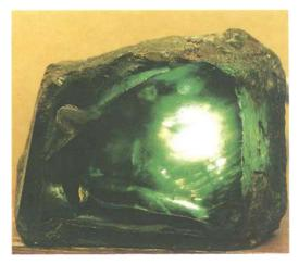
Fig. 4. A piece of metal (possibly aluminium) can be seen in the cavity in the top left-hand corner. Transmitted light.
