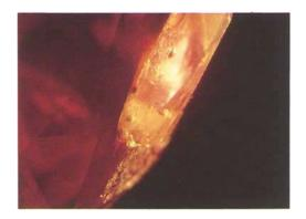
Fig. 3. Dark field illumination reveals the glassy material used to bind a small piece of natural ruby to a larger piece of synthetic ruby. Gas bubbles are visible in the glass portion while a dense white cloud of rutile silk is visible in the upper right corner of the natural piece at right. 50x. Photo by Wimon Manorotkul, AIGS.
