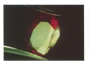
Fig. 1. Overhead lighting reveals a small piece of natural Burmese ruby (right) held to a much larger piece of Verneuil synthetic ruby (left) with glass. The slightly more dull lustre of the glass filling reveals its true nature. 10x. Photo by Wimon Manorotkul, AIGS.
