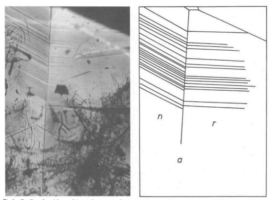
Fig. 7. Families of straight parallel growth planes in Chatham synthetic sapphire, growth sectors confined to the positive rhombohedron r(1011) [right part] and the hexagonal dipyramid n(2243) [left part] are divided by a twin boundary parallel to  $\sigma(1120)$ ; a re-entrant angle is formed by the faces n and r. Left: microphotograph, 40 x; right: drawing of growth and composition planes.
