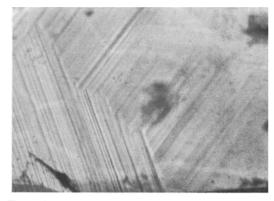
Fig. 9. Families of straight parallel growth planes that form an angle in natural ruby from Sri Lanka viewed in a direction parallel to the c-axis; planes parallel to prism faces a and a' (1120) form an angle of 120°. 30 x.
