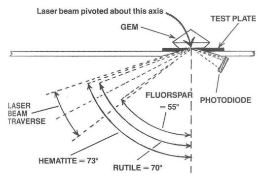
Fig. 5. Sketch showing the optics of the experimental refractometer.
