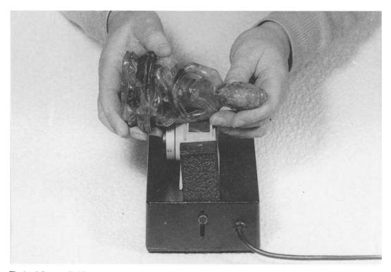
Fig. 4 A fluorspar Buddha carving on the refractometer.
