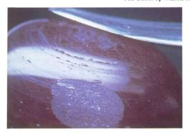
Fig. 4. Each of the cracks in this heavily included natural ruby has been filled with glass. The glass is visible with overhead lighting, due to its lower lustre. 25x. Photo by Wimon Manorotkul, AIGS.
