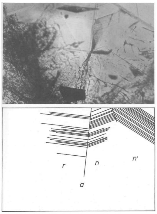
Fig. 8. Families of straight parallel growth planes in Chatham synthetic sapphire, growth sectors confined to the positive rhombohedron r(1011) [left part] and the hexagonal dipyramid n (2243) [right part] are divided by a twin boundary parallel to a (1120); a re-entrant angle is formed by the faces n and r [centre]; planes parallel to n and n' (2243) form an angle of 128° [right part]. Upper part: microphotograph, 30 x; lower part: drawing of growth and composition planes.
