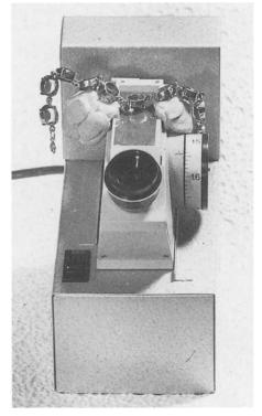
Figs. 5 and 6. Large balls of Blu-Tack are positioned on the flanks of the refractometer. These take a firm hold of the necklet and bracelet and allow them to be straddled across the prism so that one gem at a time may be carefully lowered into contact with the prism.
