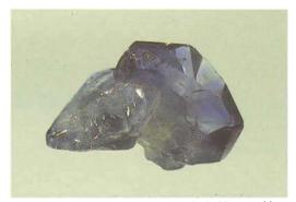
Fig. 2. Crystal group of Chatham synthetic blue sapphires, 7.02 ct in weight, consisting of two untwinned and one twinned individual. Size approx. 10 x 15 mm (photo by O. Medenbach, Bochum).
