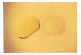
Fig. 1. Two yellow sapphires: a natural (left) and a Verneuil synthetic (right) are shown immersed in methylene iodide with diffuse light-field tungsten illumination. Due to the lack of contrast between the stone and the background, the colour zoning is difficult to see.
