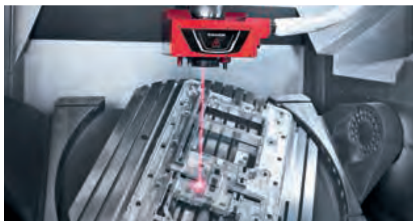
The ability of the LASERTEC 125 Shape to laser texture mould tools in five axes will replace the highly intensive and environmentally unfriendly etching process.
