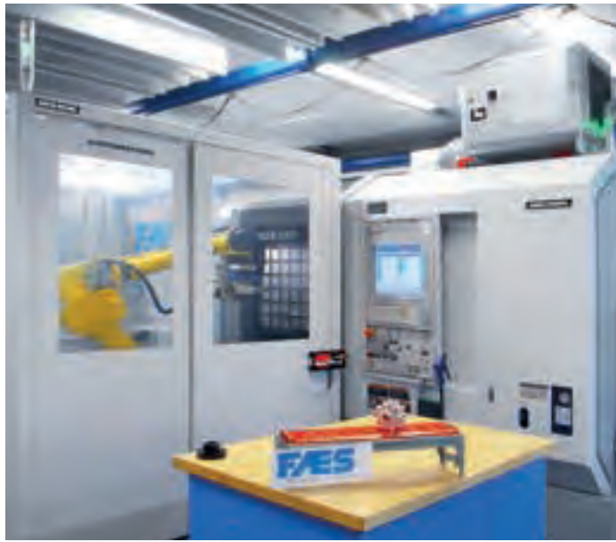
The raw and finished parts grippers of the WH25 handling robot are designed for parts weighing up to 25 kg.
