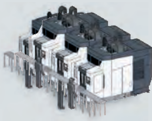
Manual transfer (Roller conveyor specification)
