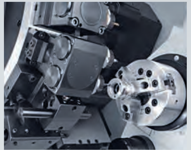
Machining of complex shapes using multi-spindle tool holders.
