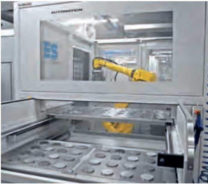
The integrated workpiece storage for parts weighing up to 300 kg guarantees safe and efficient supply of billets.
