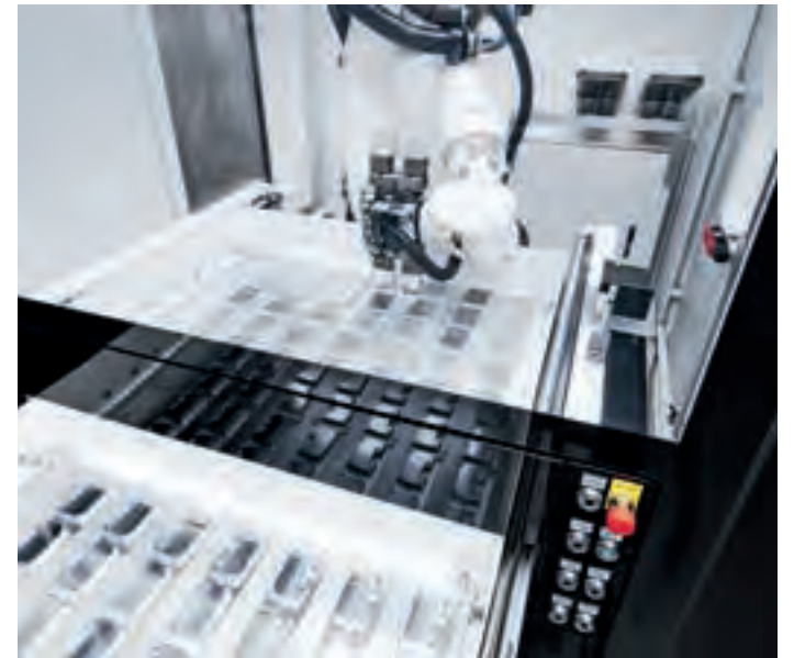
The workpiece storage with two drawers provides enough space even for extended automated operation.
