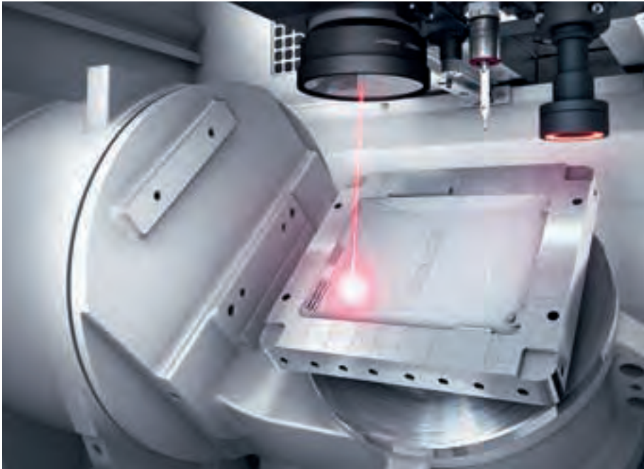
Working area of the LASERTEC 45 with integrated swivelling / rotary table (5-axis version), laser head with precision scanner, CCD camera and retractable measuring sensor.
