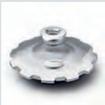
Workpiece name: Gear Material: SCM420H Size: \varnothing 80 x 40 mm Machining time: 80 sec.
