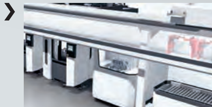
Washing Station Washing the finished cylinder block and unloading onto the conveyor.
