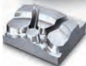
(Segment of a) tyre mould Material: SKD61 Dimensions: 190 x 170 x 70 mm Machining time: 14 hours 21 minutes Machine: NVD
