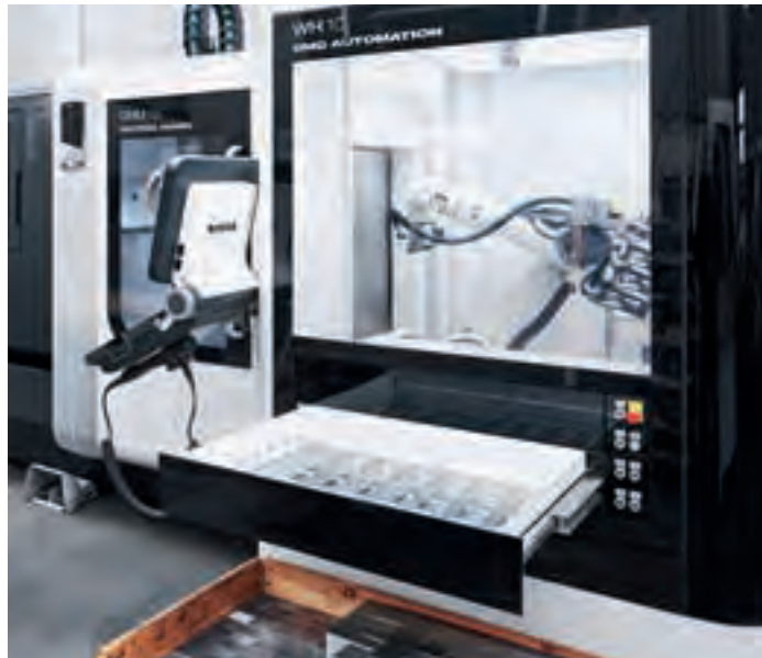
Gaiser-Mechanik can supply its customers even faster thanks to the DMU 50 with WH10 handling system.
