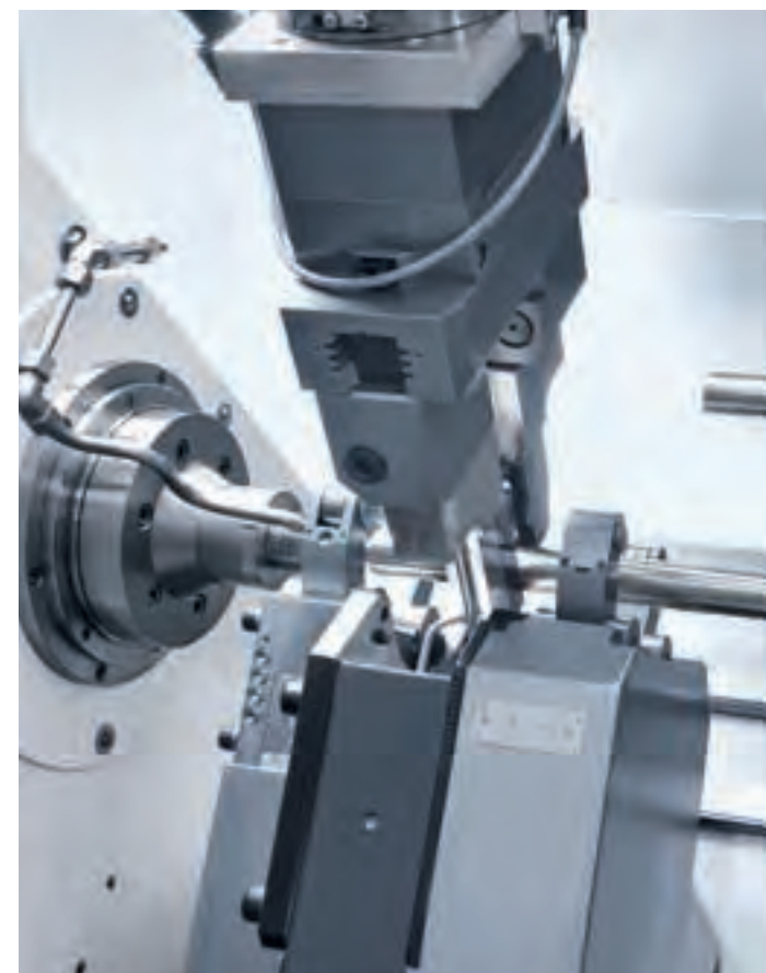
The steady rest of the CTX beta 800 linear serves to stabilise the workpiece during subsequent milling of grooves and bores.
