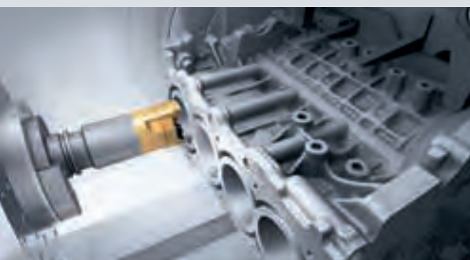
Horizontal cylinder bore machining – After tilting the A-axis table automatically, cylinder block boring follows.
