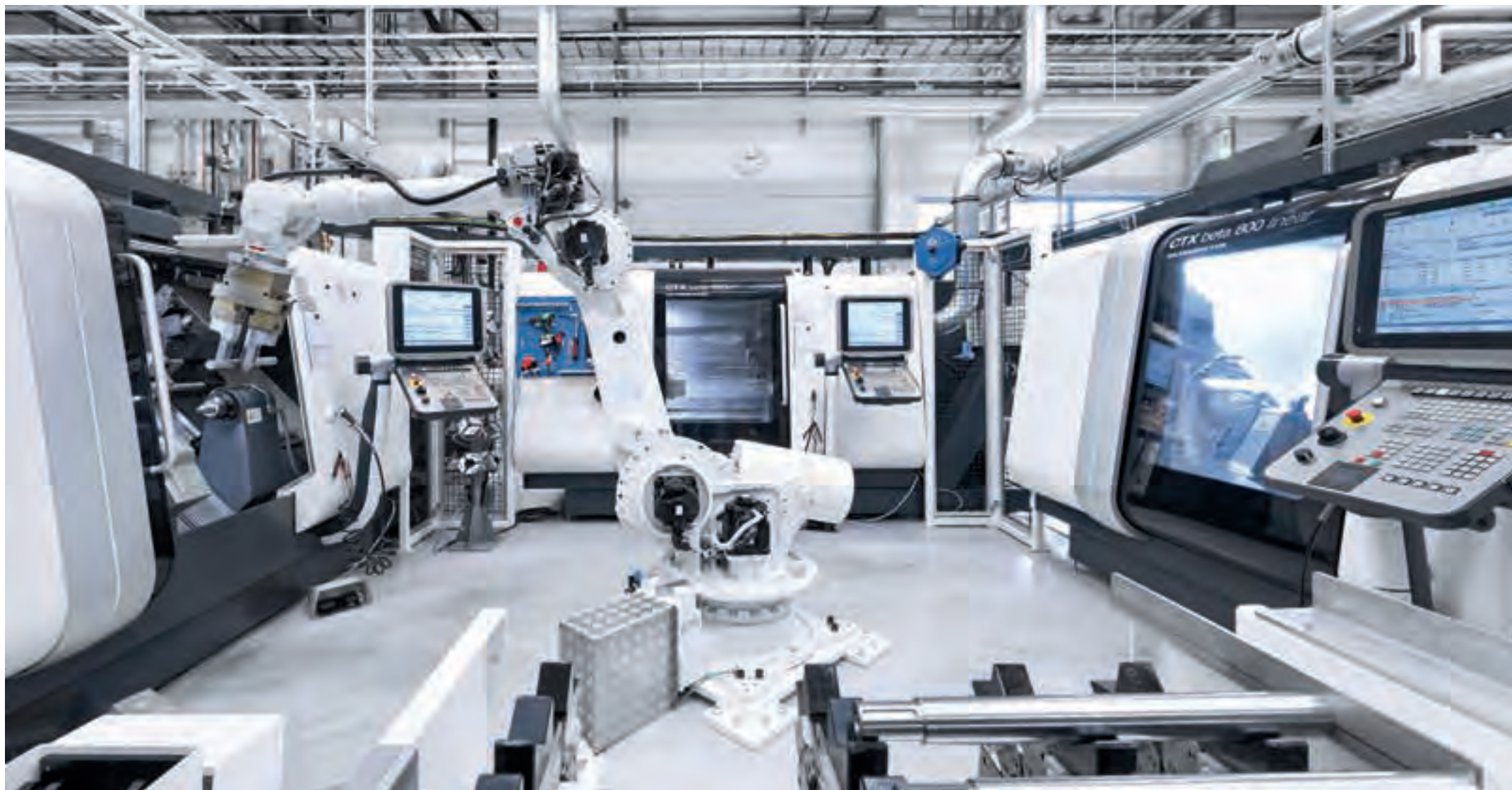
At the end of 2013 DMG MORI Systems installed a production cell at Xylem consisting of two CTX beta 800 lathes, one CTX beta 800 linear and a robot.
