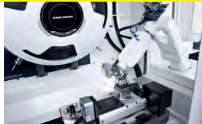
WH 2 | WH 3 workpiece handling. High degree of autonomy with short cycle times, small footprint and high workpiece storage capacity.
