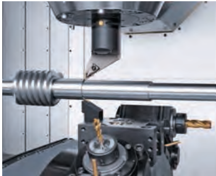
4-axis machining with B-axis and lower turret.
