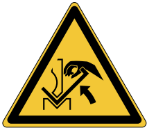
Hand crushing between press brake tool W031
