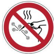
Hot works prohibited P039
