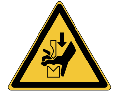
Hand crushing between press brake tool W030
