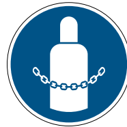
Secure gas cylinders M046
