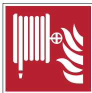
Fire hose reel F002
