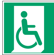
Emergency exit for people unable to walk or with walking impairment (right) E030
