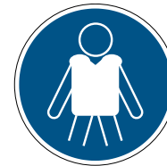
Wear personal flotation devices M053
