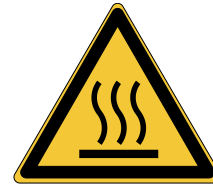
Hot surface W017
