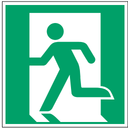
Emergency exit (left) E001
