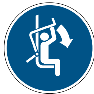
Close safety bar of chairlift M033
