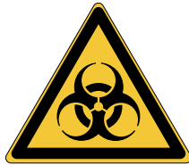
Biological hazard W009
