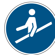
Use handrail M012
