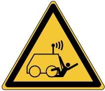
Run over by remote operator controlled machine W037
