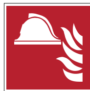
Collection of fire-fighting equipment F004
