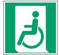
Emergency exit for people unable to walk or with walking impairment (left) E026
