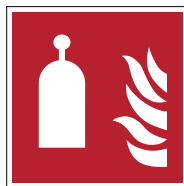
Remote release station F014
