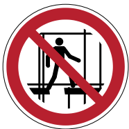
Do not use this incomplete scaffold P025
