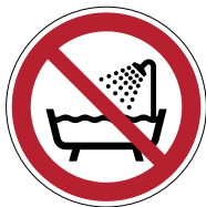
Do not use this device in a bathtub, shower or water- filled reservoir P026
