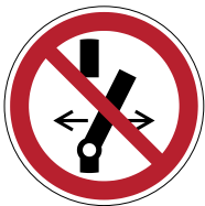
Do not alter the state of the switch P031
