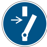
Disconnect before carrying out maintenance or repair M021
