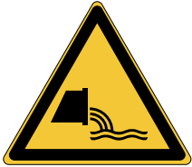
Warning Sewage effluent outfall W055
