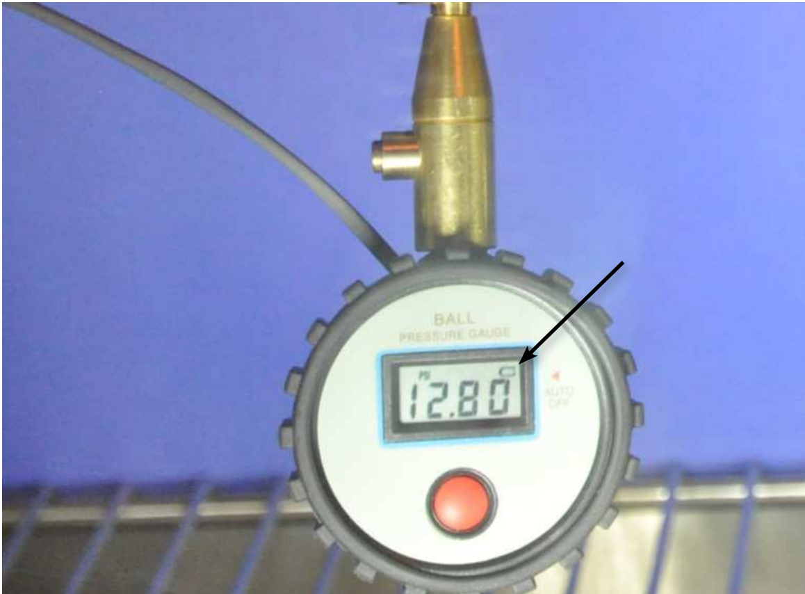
Figure 10. Close-up image of the Exemplar Gauge showing battery indicator (indicated by the arrow) on the LCD screen. The battery indicator is illuminated when the applied voltage is approximately 2.6V or less.
