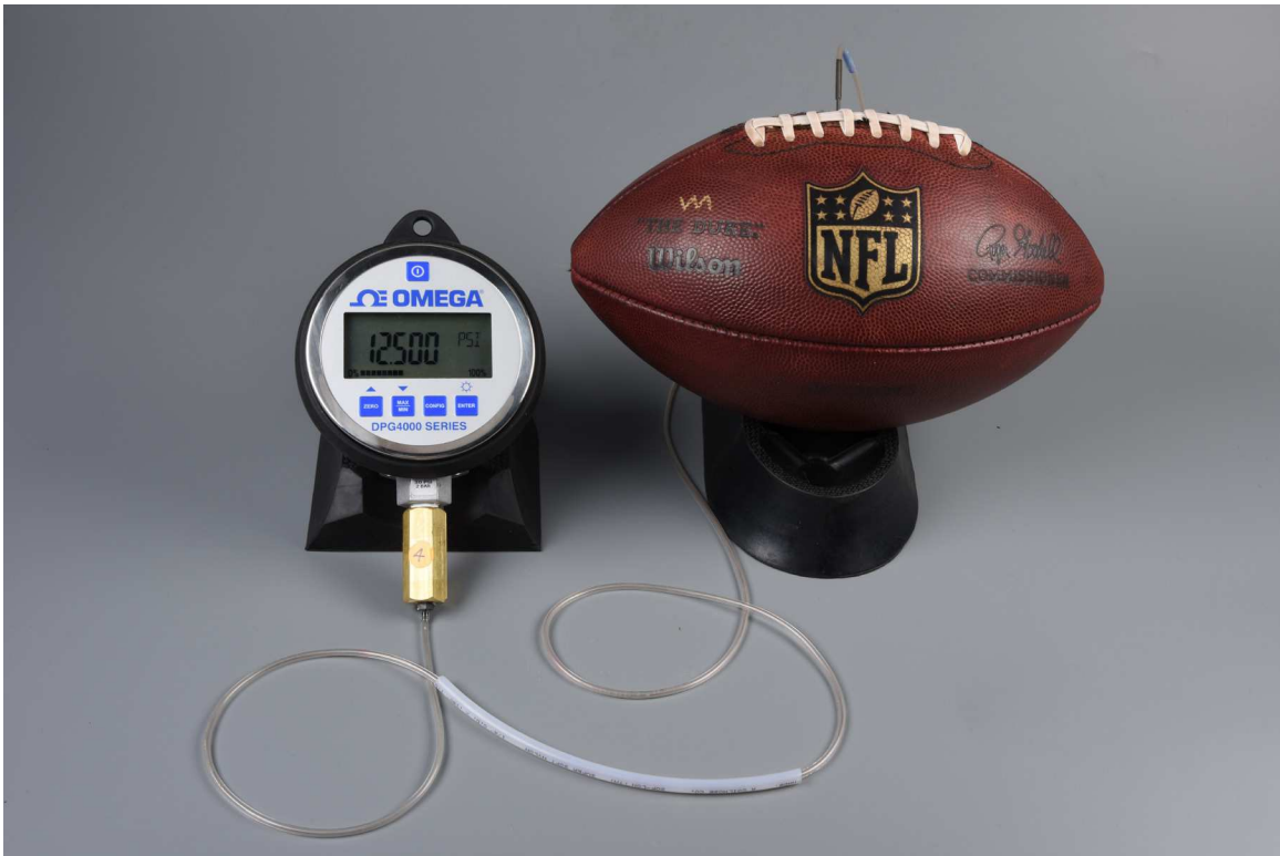
Figure 20. Photograph of the inflation needle inserted into a football. The needle remained inside the football through the transient data capture process.
