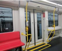
Each LRV is electrically powered from an overhead catenary system (OCS) and for San Francisco operates at speeds up to 50 mph, carrying close to 192 passengers in each vehicle with the ability to operate in multiple vehicle consists (up to four). These light rail vehicles remove automobiles off the road, in turn helping cities decrease their CO2 emissions.
