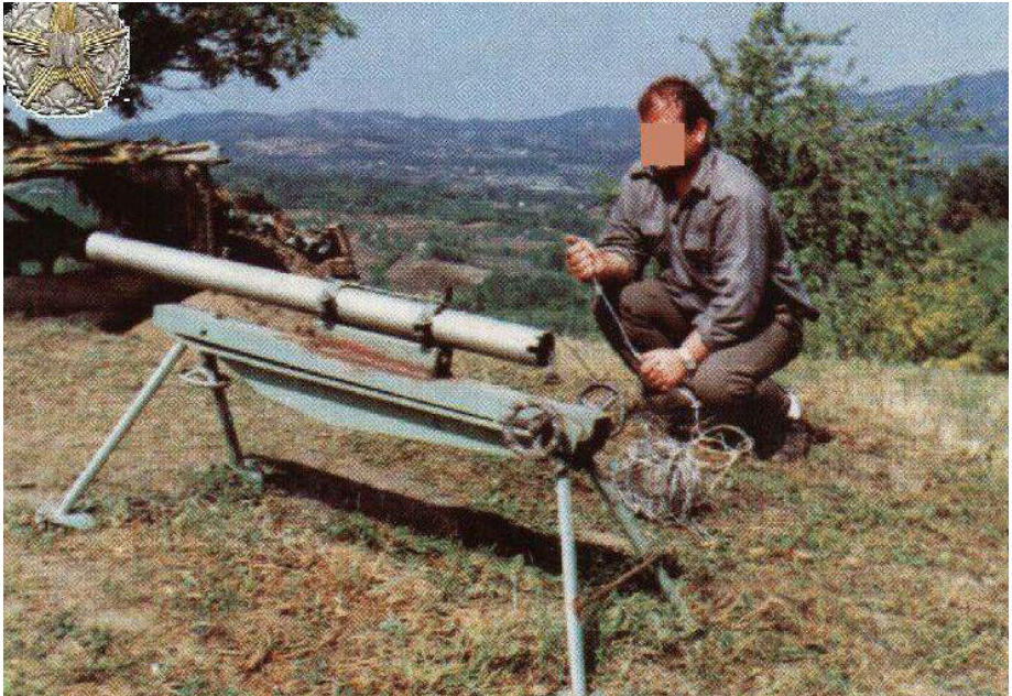
Photo 10 Portable single-tube launcher for 57 mm rockets from an unknown party to the conflicts in the former Yugoslavia in the 1990s. This launcher appears to be based around a single launch tube removed from a standard rocket pod.
