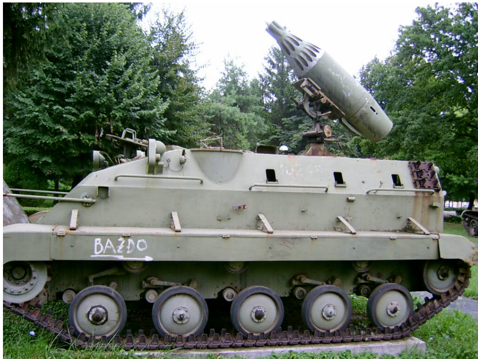
Photo 7 A modified Yugoslavian produced M-60P armoured personnel carrier (APC) with a UB-32-57 rocket pod. This vehicle was pictured at Kozare Museum (Muzej Kozara) in Banja Luka, Bosnia and Herzegovina.
