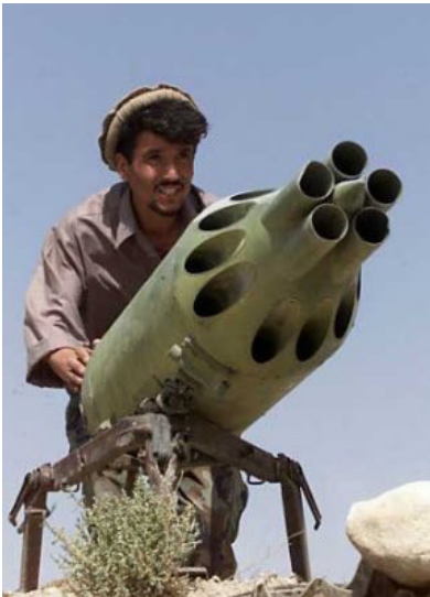
Photo 14 and 15 Improvised rocket systems based on UB-16-57 launchers in Afghanistan in the late 1990s or early 2000s.
