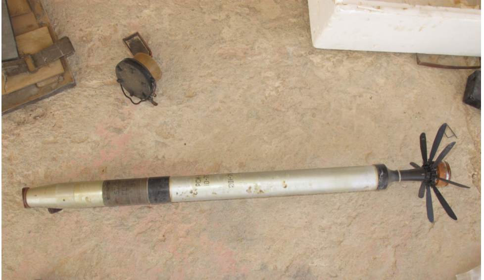
Photo 1 A 57 mm S-5KO HEAT-FRAG unguided air-to-surface rocket in Libya.
