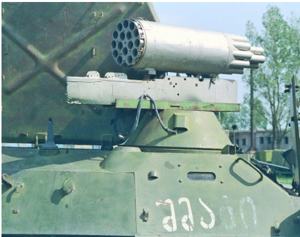
Photo 13 MT-LB multipurpose armoured vehicle with UB-16-57 rocket pod. Photo taken in Kutaisi, Georgia in 1998.
