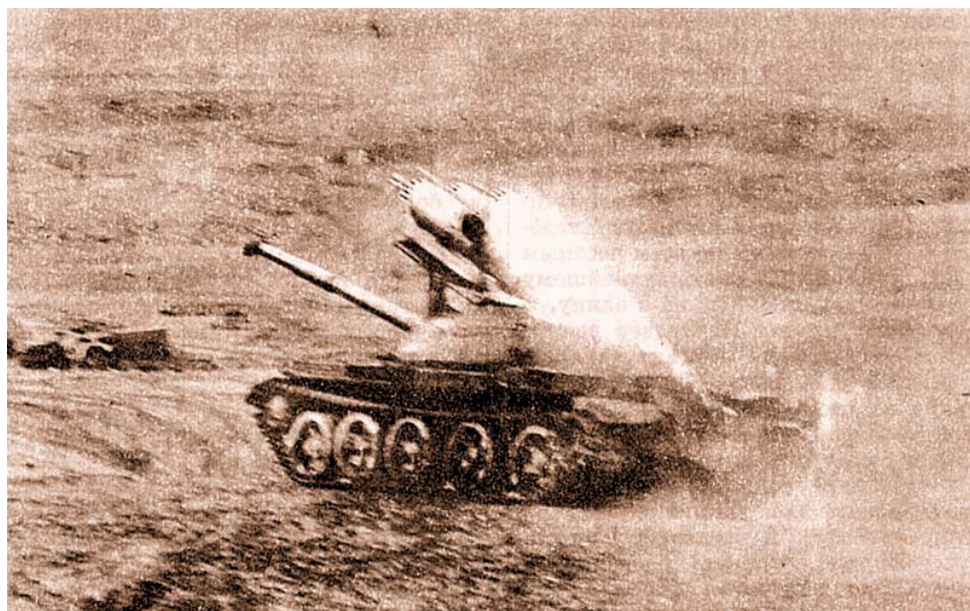
Photo 3 Soviet T-62 MBT in Afghanistan in the 1980s, with three UB-32-57 launchers mounted on an improvised platform above the turret.
