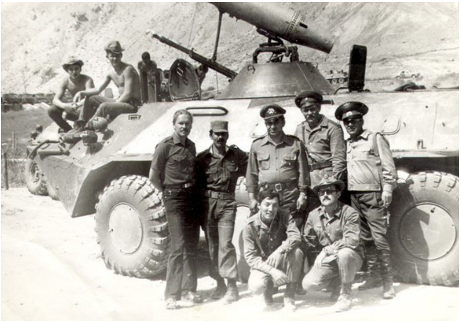
Photo 5 Soviet BTR-70 IFV in Afghanistan in the 1980s, with a UB-16-57 rocket pod in an improvised mount about the turret. From photo archive of Aksenenko Sergei, commander of the 3 rd Battalion, 122nd Regiment of the 201st Motorized Rifle Division, Soviet 40 th Army in Afghanistan from 1982-84.
