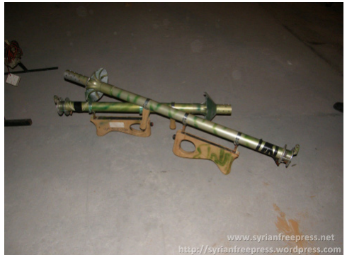
Photo 16 and 17 Improvised man-portable, shoulder-fired single-tube rocket launcher for 57 mm S-5 rockets. Photos were taken after the discovery of a large consignment of weapons, allegedly smuggled out of Libya in 2012 aboard the ship Letfallah II.
