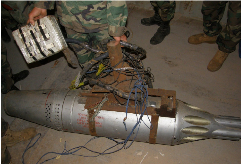
Photo 2 A UB-16-57 rocket pod capable of being loaded with up to 16 S-5 rockets of 57 mm, and its improvised firing system. Photos were taken after the discovery of a large consignment of weapons, allegedly smuggled out of Libya in 2012 aboard the ship Letfallah II. Photo credit: Syrian Free Press
