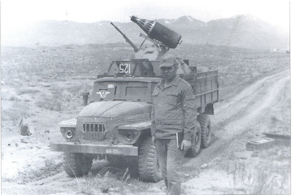
Photo 4 Soviet Ural 4320N truck in Afghanistan in the 1980s, with a UB-32-57 rocket pod mounted atop an improvised conversion of a BRDM-2 turret.
