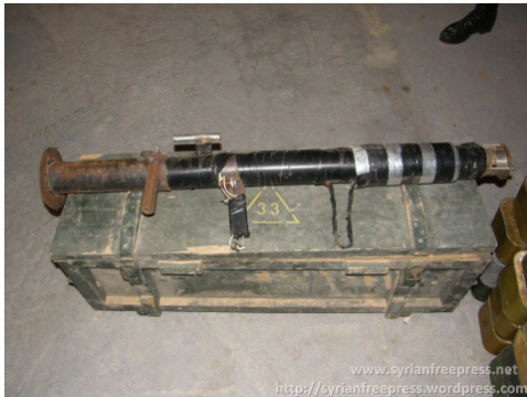
Photo 16 and 17 Improvised man-portable, shoulder-fired single-tube rocket launcher for 57 mm S-5 rockets. Photos were taken after the discovery of a large consignment of weapons, allegedly smuggled out of Libya in 2012 aboard the ship Letfallah II.
