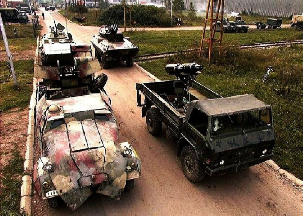
Photos 8 and 9 A TAM-110 truck operated by Republika Srpska forces in Bosnia and Herzegovina in the mid-1990s, fitted with two UB-16-57 rocket pods. Photo credit: UK Ministry of Defence
