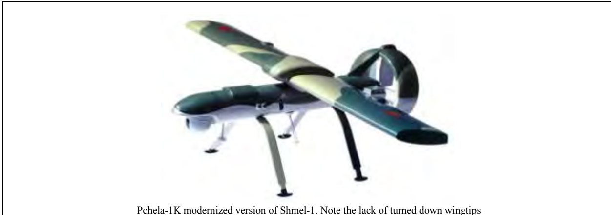
Pchela-1K modernized version of Shmel-1. Note the lack of turned down wingtips
