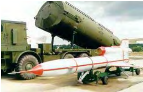
Tu-143 on transporter-erector-launcher (TEL)
