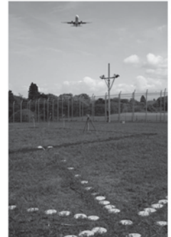
Fig.1 Noise source distribution measurement at Narita Airport
